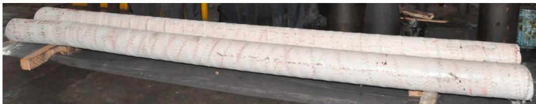
Figure 3.3: 230 mm diameter double stage radially forged zr-2.5Nb alloy ingots
