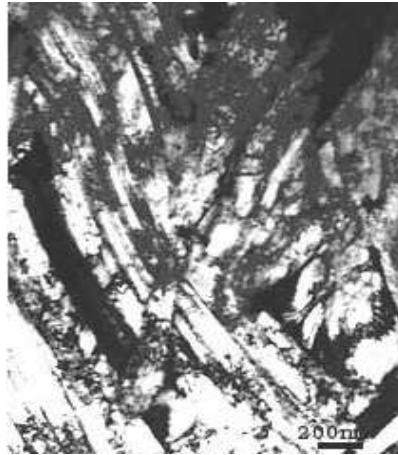
Figure 5.10: TEM longitudinal micrograph after second pass pilgering
