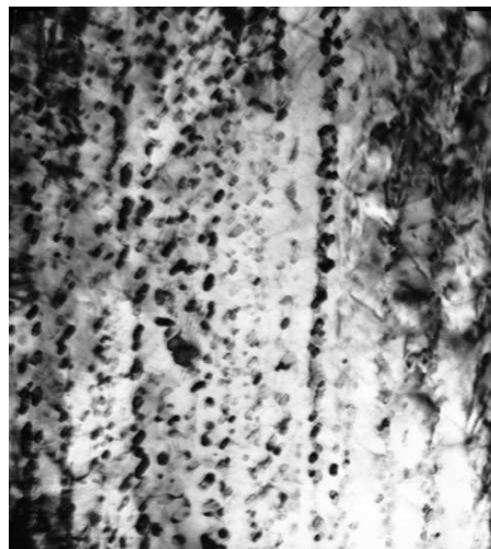
Figure 5.13: TEM micrographs after Autoclaving (290°C/120 hrs)
