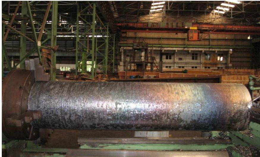
Figure 3.1: Quadruple melted Ingot by VAR melting method
