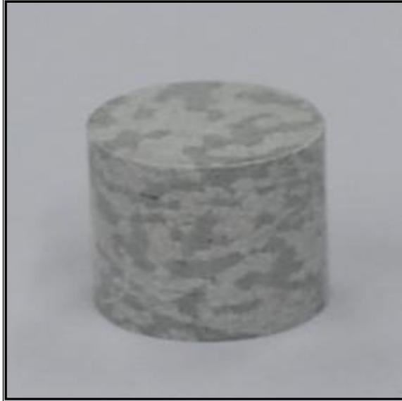
**Figure 3.6:** *ThO<sub>2</sub>-5%CeO<sub>2</sub> green pellet fabricated by CAP process.*
