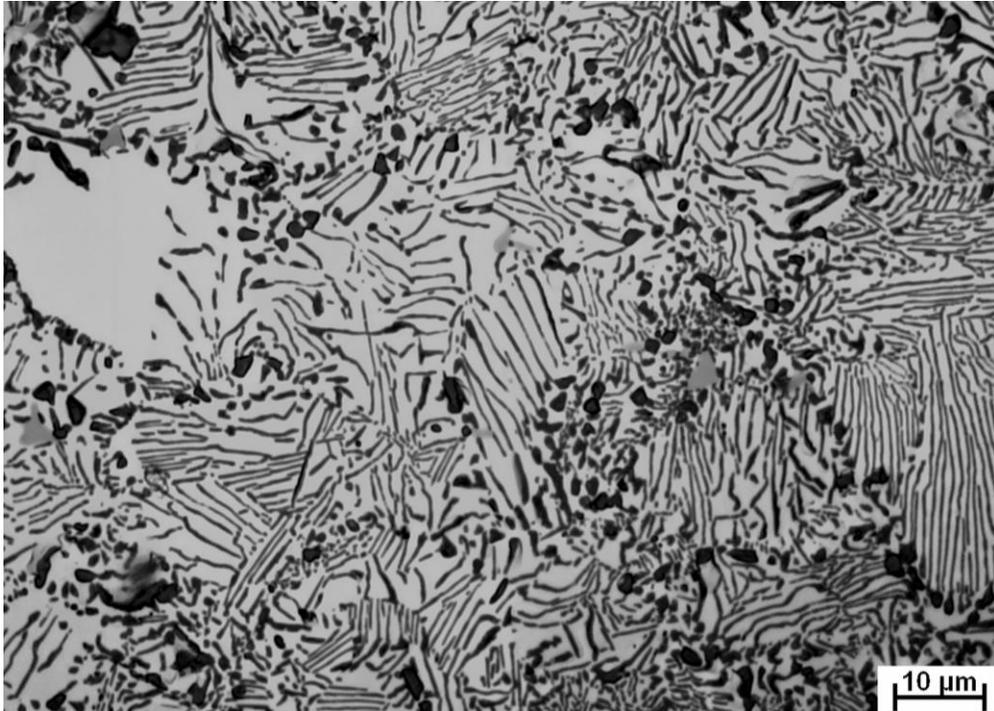
**Figure 5.12** Optical micrograph of as-rolled U-9 wt.% Mo alloy after ageing at 565 °C for 14 days.
