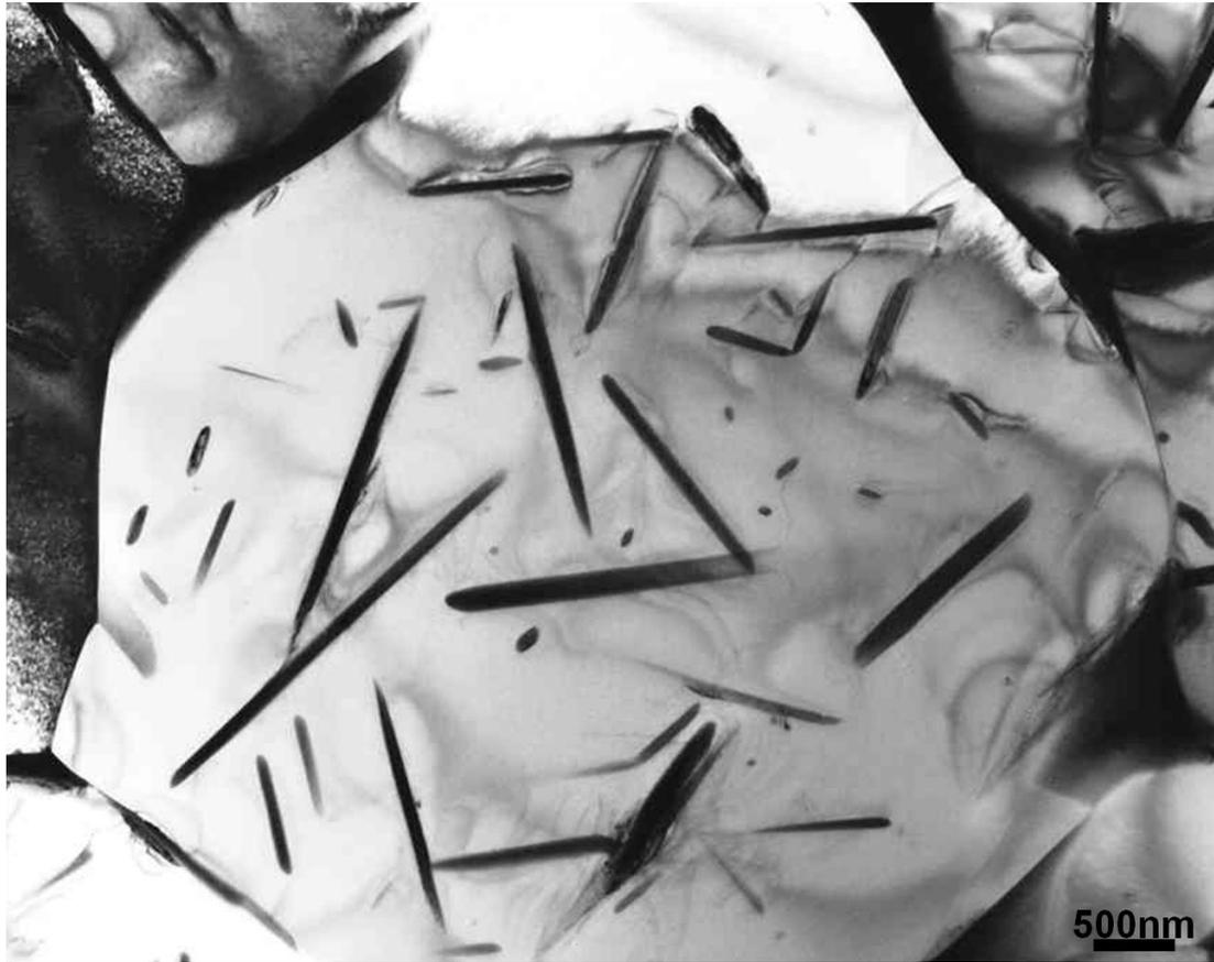
**Figure 4.5** A typical bright-field TEM micrograph representing the microstructure of Zr-1 wt.% Nb alloy sample heat treated at 825 °C for 10 mins.
