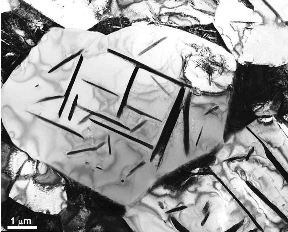
**Figure 4.6** A typical bright-field TEM micrograph representing the microstructure of Zr-1 wt.% Nb alloy sample heat treated at 832 °C for 5 mins.
