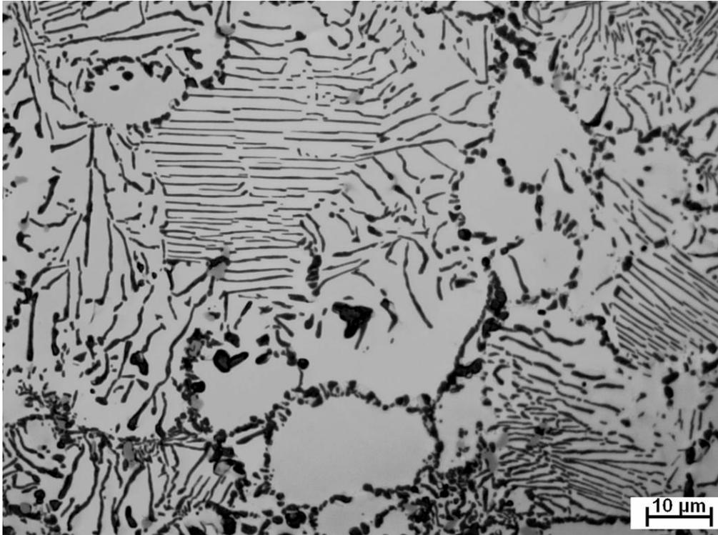
*Figure 5.11* Optical micrograph of as-rolled U-9 wt.% Mo alloy after ageing at 565 °C for 7 days.
