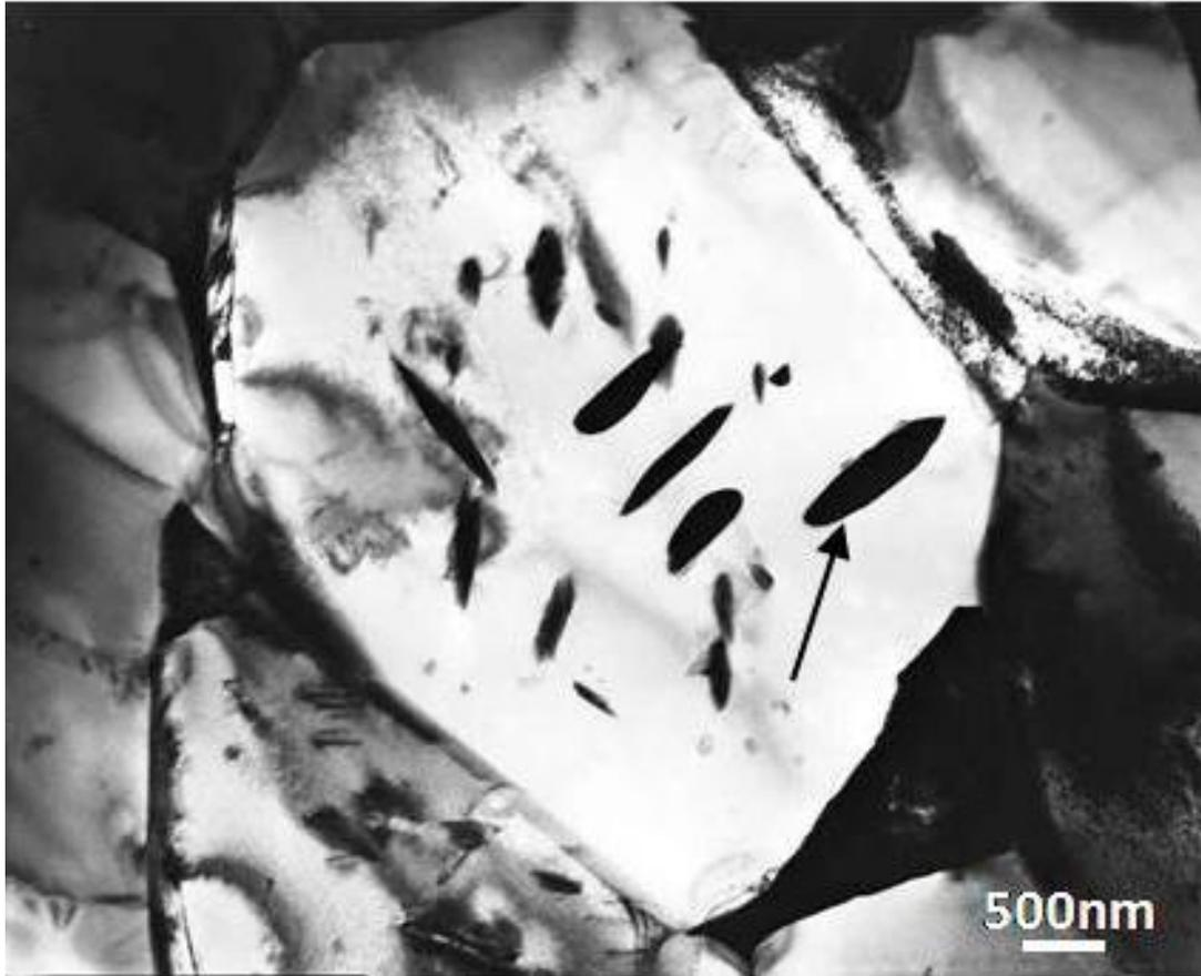
**Figure 4.11** Bright-field TEM micrograph showing the  $\beta$ -precipitate in the Zr-1 wt.% Nb alloy sample heat treated at 800 °C for 30 mins (marked by an arrow) from which the SAED patterns in Figure 4.10 are obtained.
