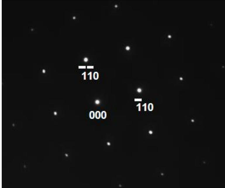
**Figure 5.4** A typical SAED pattern (Zone Axis =  $[001]_{\gamma}$ ) obtained from the  $\gamma$ -phase present in the microstructure of the as-rolled U-9 wt.% Mo alloy sample furnace-cooled after being homogenized at  $1000^{\circ}\text{C}$  for 24 h.
