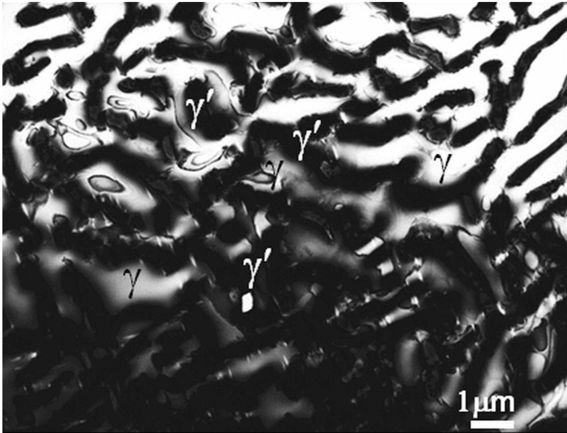
**Figure 5.24** A typical bright-field TEM micrograph showing the partially decomposed type-III ( $\gamma + \gamma'$ ) lamellar colony comprising of short  $\gamma'$ -phase lamellae and  $\gamma$ -interlamellar regions in U-9 wt.% Mo alloy.
