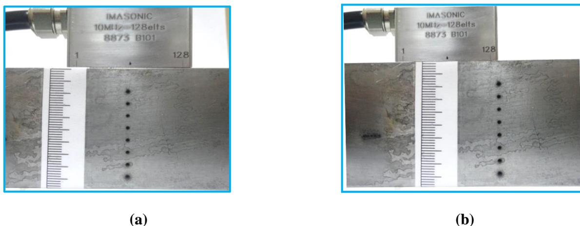
**Figure 5.1: Experimental set-up for detection and characterization of vertically stacked holes in carbon steel sample (a) SFLA, PA-SAFT and FMC techniques (b) Conventional angle beam phased array using focal laws (Scale in mm)**
