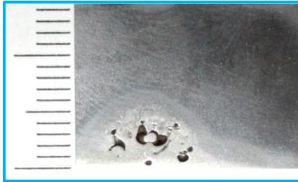
**Figure 6.3: Clustered porosity in the weld sample (Scale in mm)**
