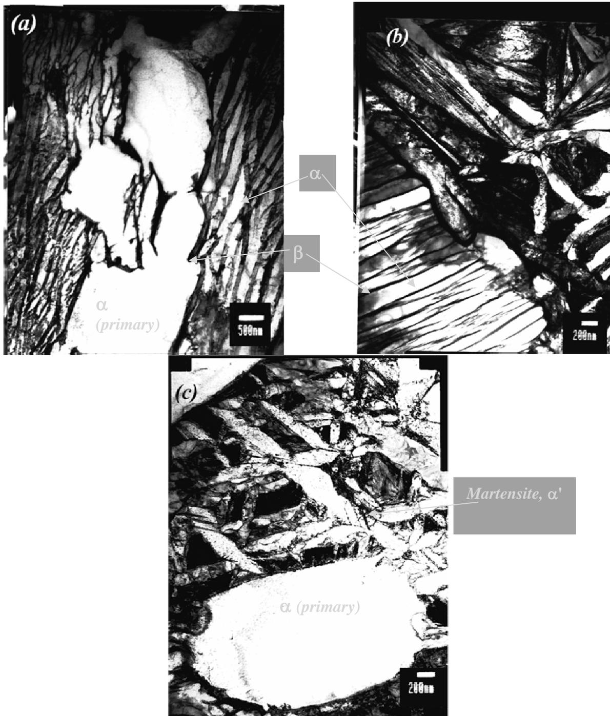
Fig. 4.7 Bright field TEM micrographs showing distribution and morphology of primary  $\alpha$  and  $\beta$ -phase transformed products  $\alpha$ ,  $\beta$  and  $\alpha'$  for the samples soaked  $870\pm 0.5^\circ\text{C}$  and cooled at, (a)  $10^\circ\text{C/s}$ , (b)  $25^\circ\text{C/s}$  and (c)  $50^\circ\text{C/s}$
