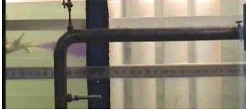
**Figure 4.15: Full scale poison jet facility-Jet cross first row of calandria tubes**
