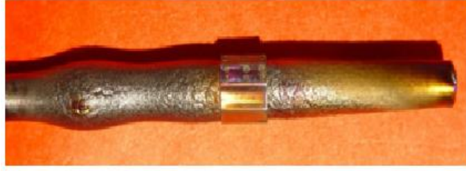
Figure 2.3: Ballooned Fuel Pin [8]
