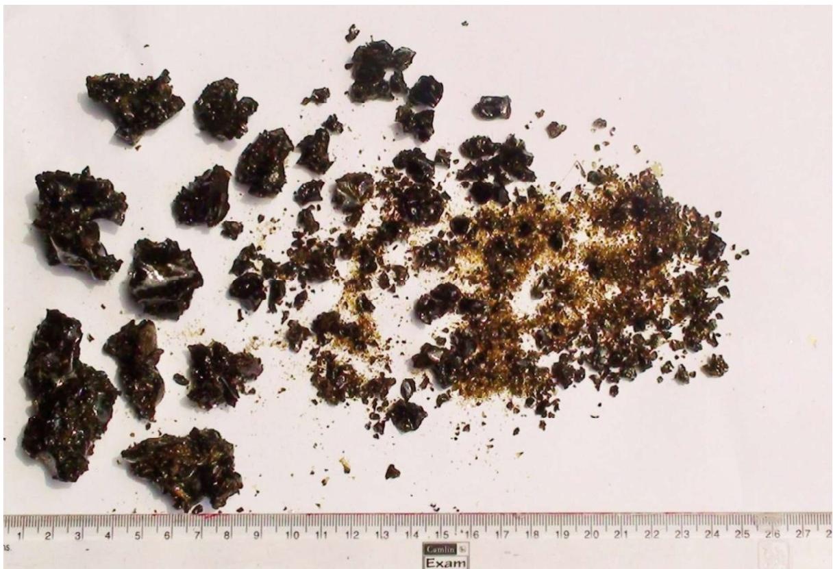
Figure 25: Porous mass and debris size in bottom flooding experiment
