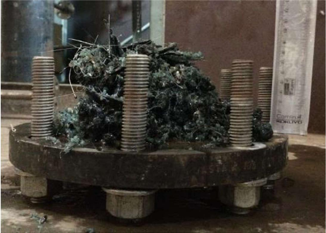
*Figure 82: Debris obtained from experiment with  $M/W=0.21$*
