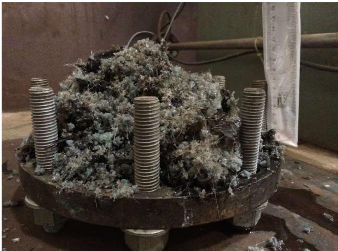
Figure 84: Debris obtained from experiment with  $M/W=0.41$
