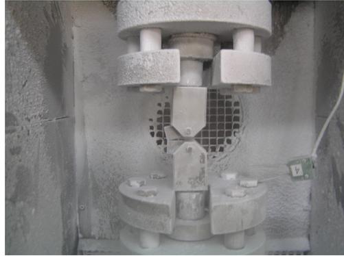
FIGURE 5.3: 0.4T CT specimen tested at sub-zero temperature in environmental chamber using UTM
