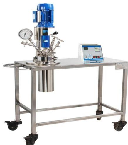
**Fig.3.6: Trolley mounted autoclave**
