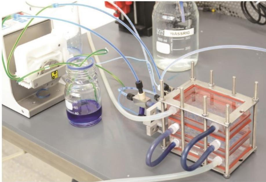
**Figure 1.15:** Two-stage counter-current setup (Holbach and Kockmann, 2013)
