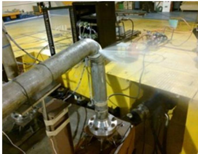
Figure 2.12: Water jet through crack at crown of SSPS elbow
