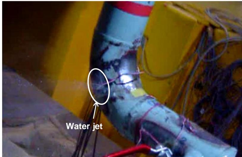
Figure 4.16: Water jet through crack at crown of elbow
