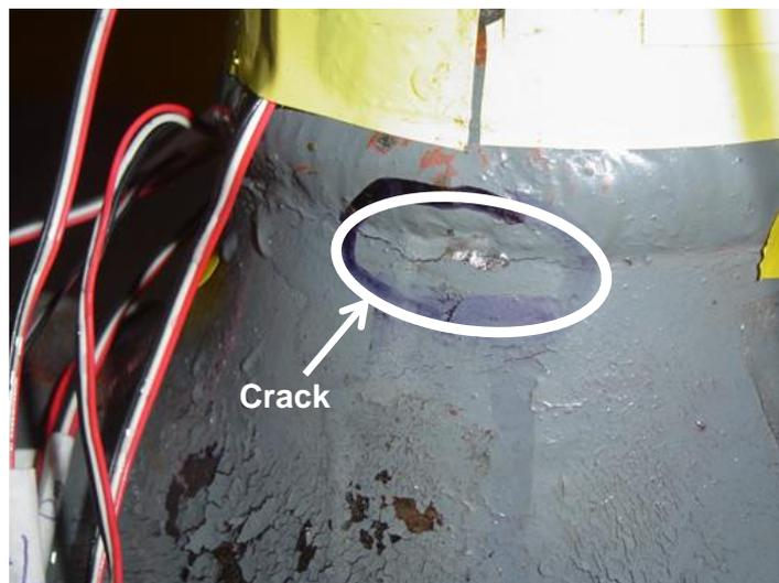
Figure 4.17: Crack at the weld location of tee and pipe
