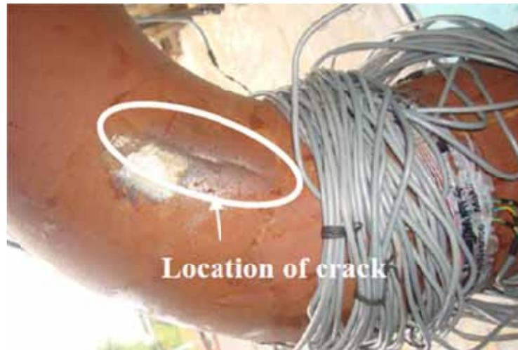
Figure 5.21: Photograph of crack at crown of the elbow
