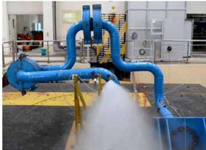
Figure 5.9: Photograph of rupture at crown
