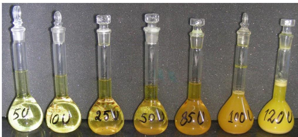
*Figure 6.2: Uranyl nitrate solution prepared in 3M nitric acid at various uranyl nitrate concentrations. The respective systems are marked on the round bottom flask indicating the concentration of uranyl nitrate.*
