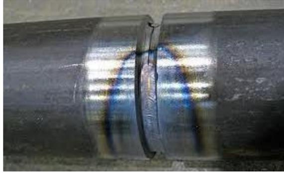
**Fig.2.1: weld distortion in a circumferential pipe joint**
