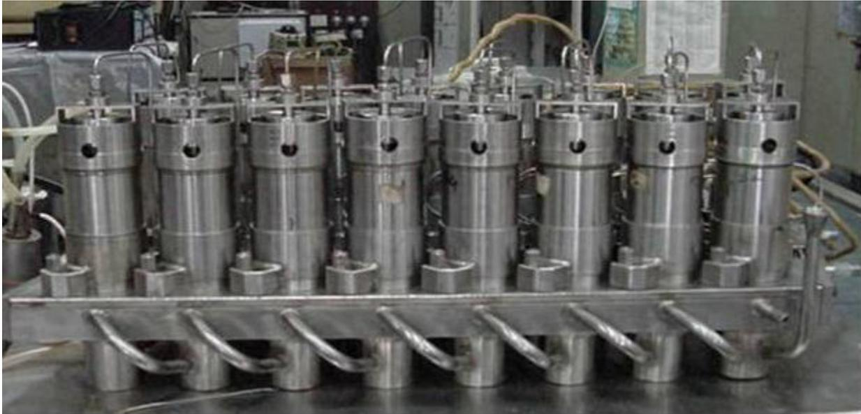
**Fig. 1.2: A typical View of 16-stage Centrifugal extractor bank**
