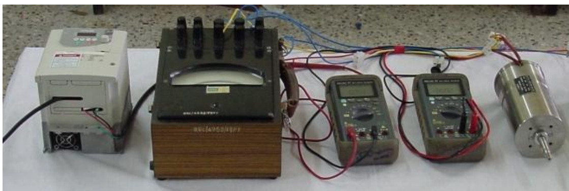
Fig. 4.5 Test set up for induction motor.
