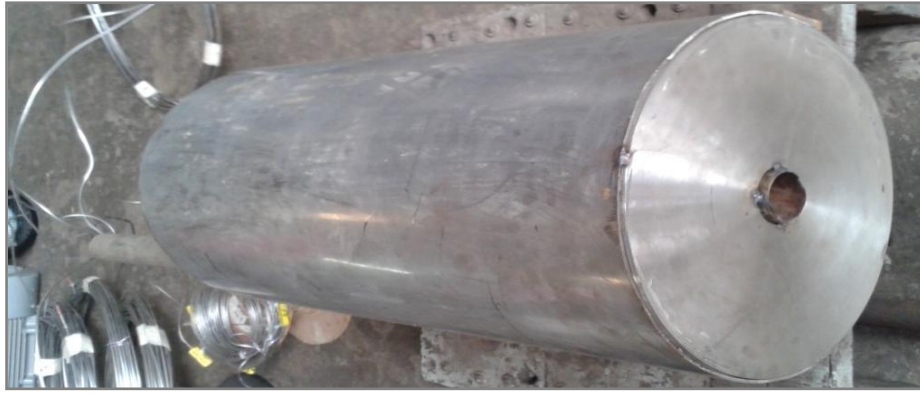
Fig.4.25 Manufactured submersible ALIP with outer stainless steel enclosure
