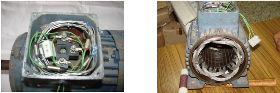
Fig. 4.20 Conventional motor winding replaced with MI cable winding
