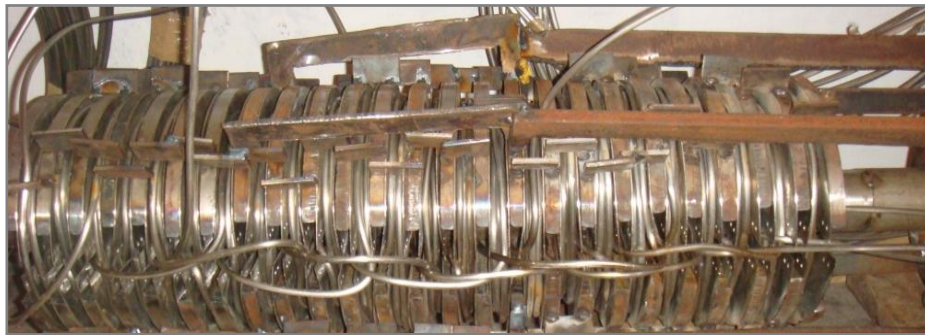
Fig. 4.23 MI cable winding of submersible ALIP along with fixtures and support
