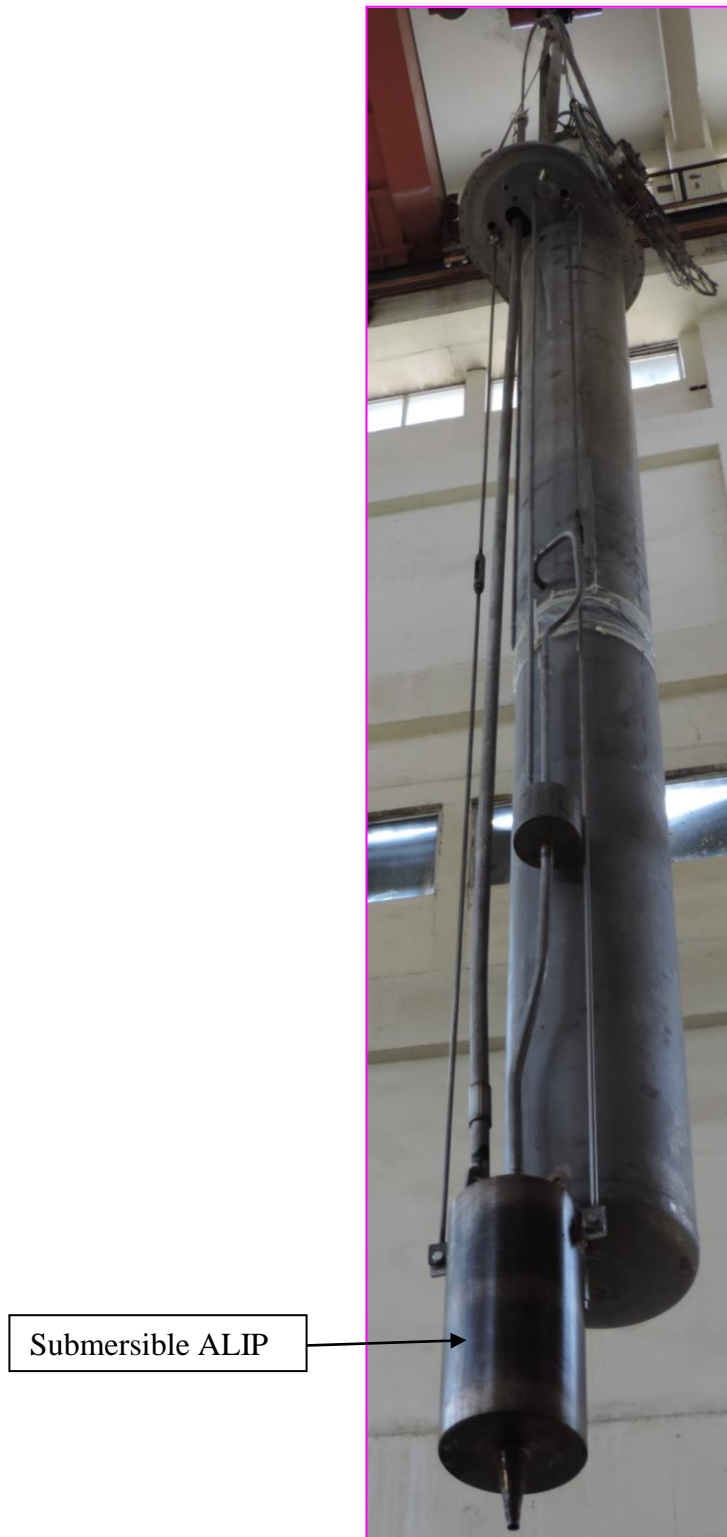
Fig. 5.18 Erection of submersible ALIP for testing in ICT
