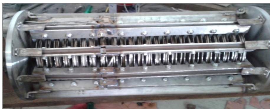
Fig.4.24 Submersible ALIP with MI Cable winding and CRGO laminations
