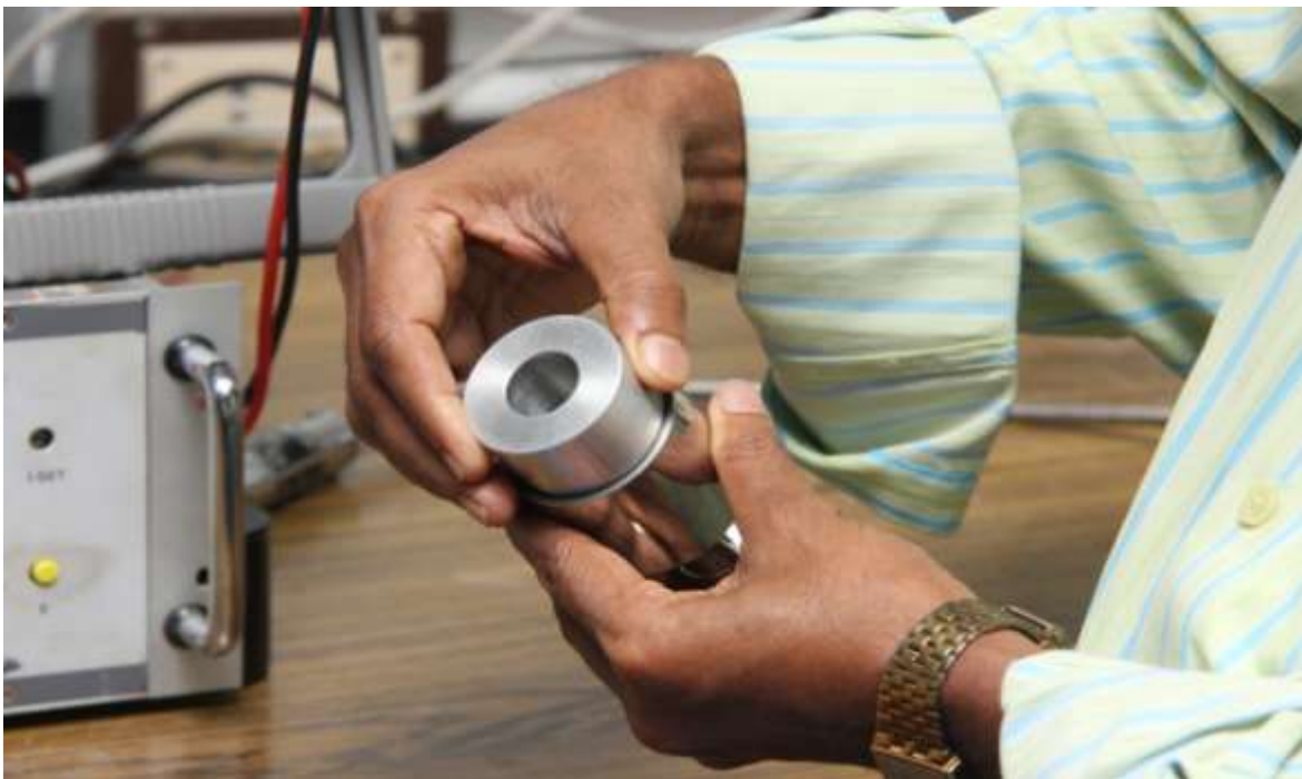
Fig. 2.20: Simulated checking of the developed probe with aluminium block
