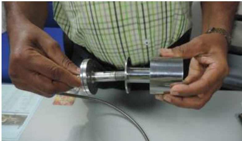
Fig.2.25: Miniature detector for FBTR
