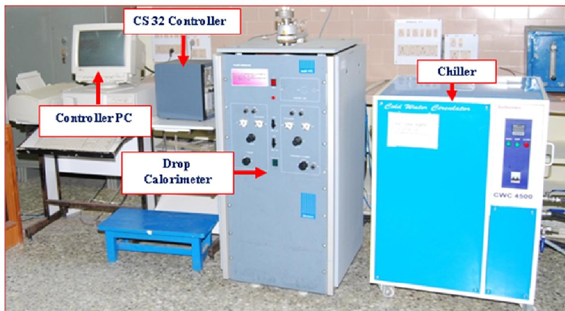
**Fig. 2.8.** The experimental setup of inverse drop calorimeter used in the present study
