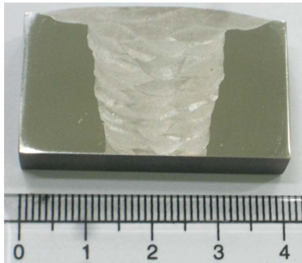
Fig. 2.4 Weld joint specimen used in ABI test.
