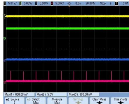
(b) Output voltages of flip flops:  $Q_1$  (yellow) is at 0 V,  $Q_2$  (green) is at 5 V,  $Q_3$  (blue) is at 0 V and clock signal (pink)
