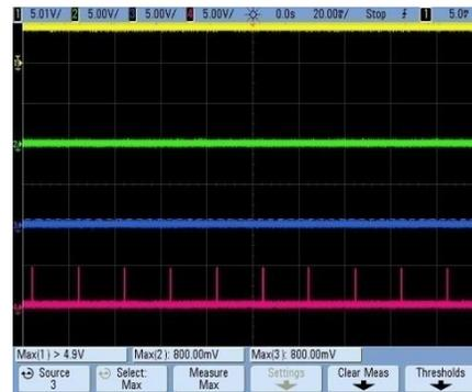
(b) Output voltage of flip flops:  $Q_1$  (yellow) is at 5 V,  $Q_2$  (green) is at 0 V,  $Q_3$  (blue) is at 0 V and clock signal (pink)
