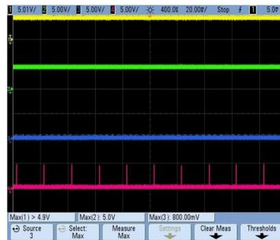
(b) Output voltage of flip flops:  $Q_1$  (yellow) is at 5 V,  $Q_2$  (green) is at 5 V,  $Q_3$  (blue) is at 0 V and clock signal (pink)
