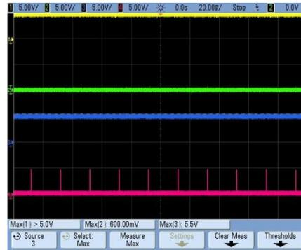
(b) Output voltage of flip flops:  $Q_1$  (yellow) is at 5 V,  $Q_2$  (green) is at 0 V,  $Q_3$  (blue) is at 5 V and clock signal (pink)
