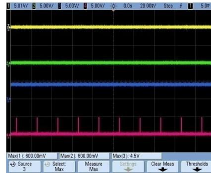
(b) Output voltage of flip flops:  $Q_1$  (yellow) is at 0 V,  $Q_2$  (green) is at 0 V,  $Q_3$  (blue) is at 5 V and clock signal (pink)
