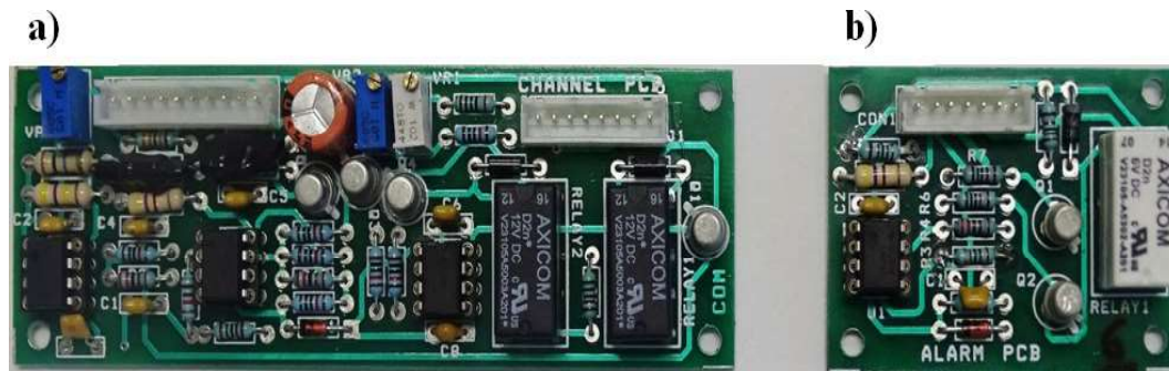
Figure 5.9. Developed PCBs a) Early fault detection with channel loop functional test PCB for each channel and b) early fault detection PCB for alarm module.
