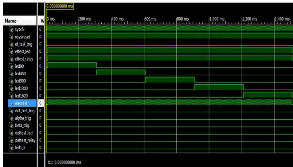
Figure 6.10. Simulation output of iSim during AGRM electronic test with a frequency of 1 GHz. The design signals, test trigger input, LED indication, GM tube isolation relay activation and test frequency output are shown.
