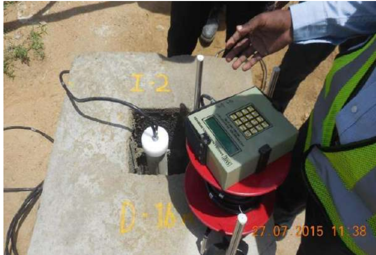
Fig 4.6: Assembly of inclinometer and read out unit at location I2.
