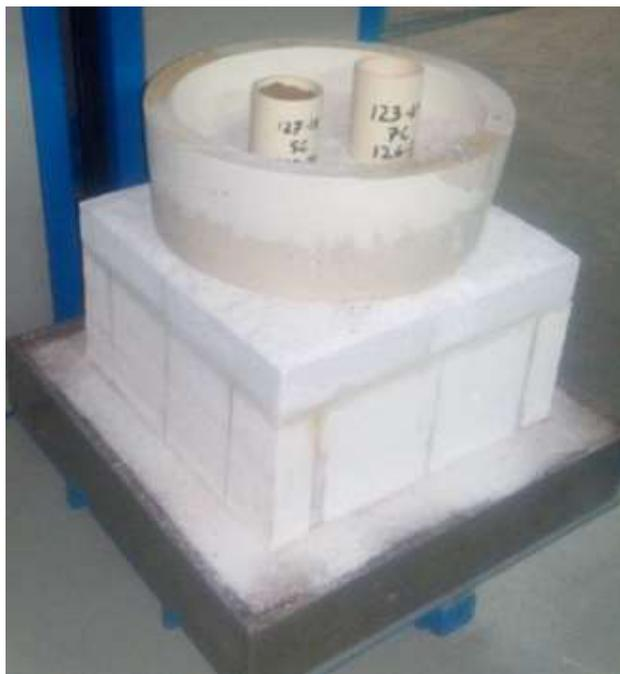
**Figure 3.2:** Dilatometer for measuring coefficient of thermal expansion of glass
