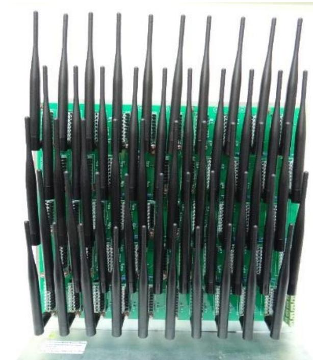
Figure 4-17: Fabricated 5 × 10 array rectenna panel with antenna
