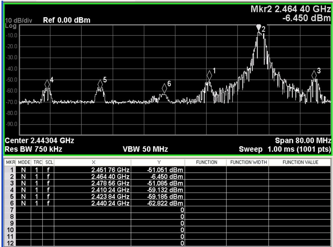
Figure 3-14: RF signal captured through SA for Design-2
