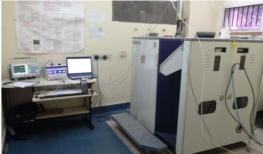
**Figure 5.4. Irradiation experimental setup at gamma chamber -5000**
