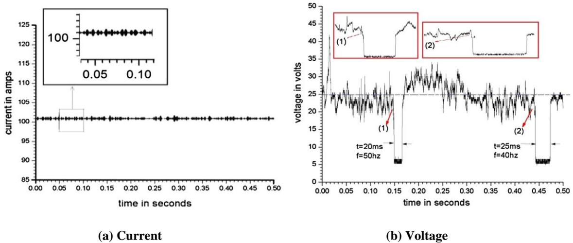
**Fig. 4.17: Voltage and current signature pattern using E 7018 electrode and inverter power supply.**
