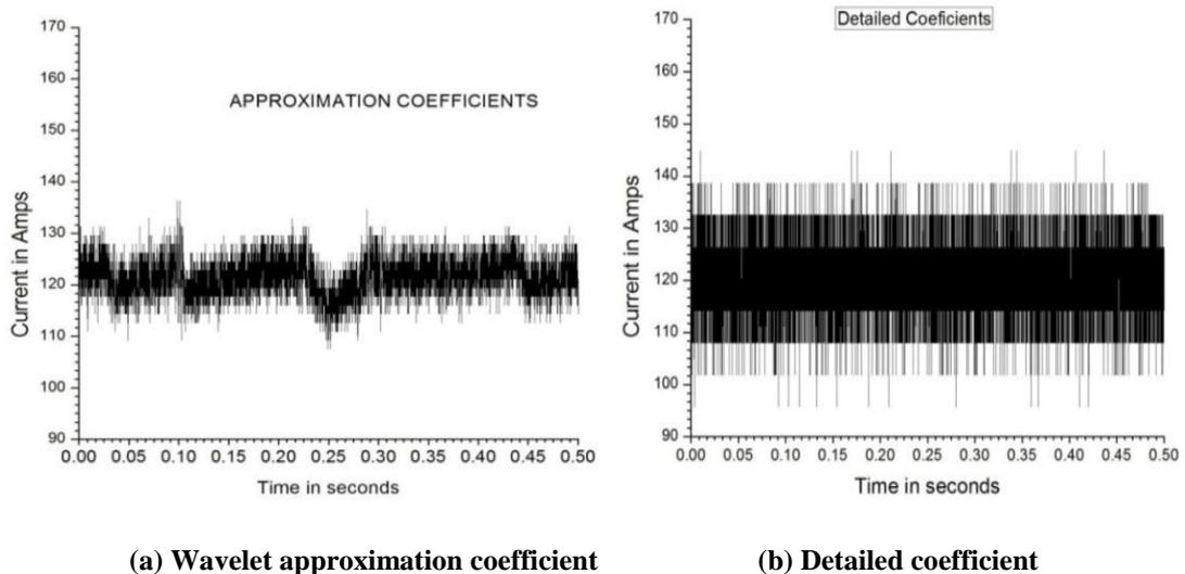
**Fig. 3.5: Samples of filtered welding current with DWT filtering techniques (a) with wavelet approximation coefficient and (b) with detailed coefficient.**
