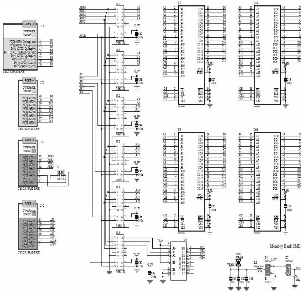
Fig. 5.8: Memory addressing arrangement in PSoC-5 based design.
