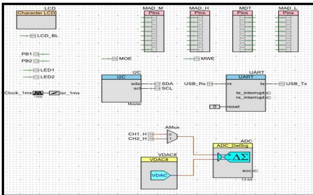
**Fig. 5.5: Top schematic of PSoC-3 based design.**
