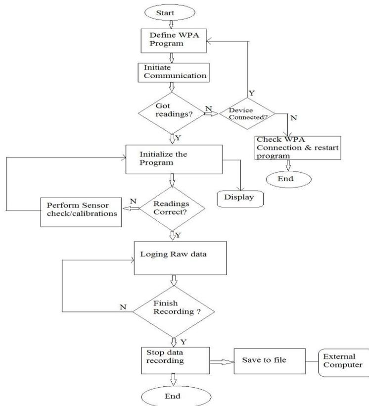
Fig. 5.11: Working flow diagram of WPA.
