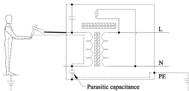
**Fig. 2.7: Torch Current between welding circuit connections and PE.**
