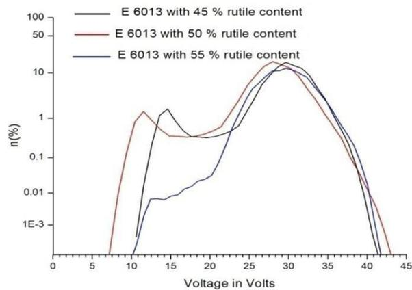
**Fig. 4.26: PDD analysis of E 6013 electrode with varying rutile content.**
