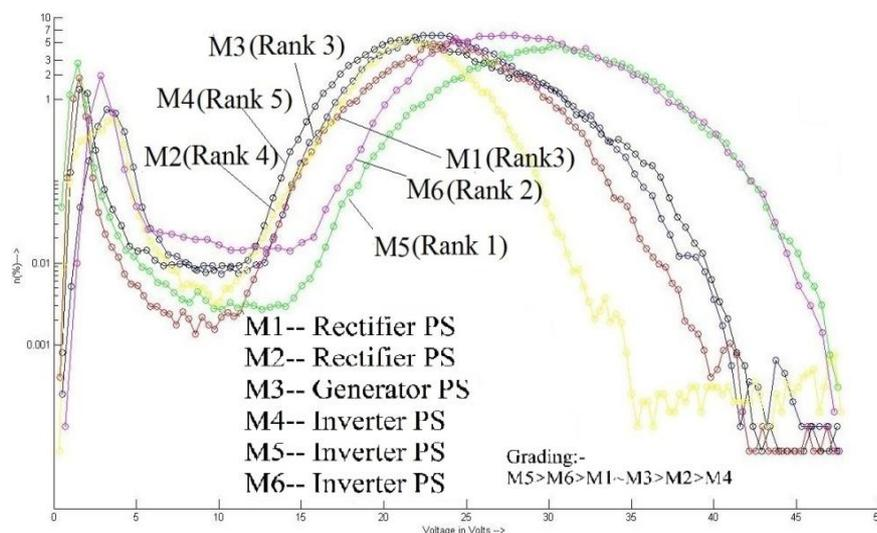
**Fig. 4.13: Voltage and current PDDs of various welding power sources.**
