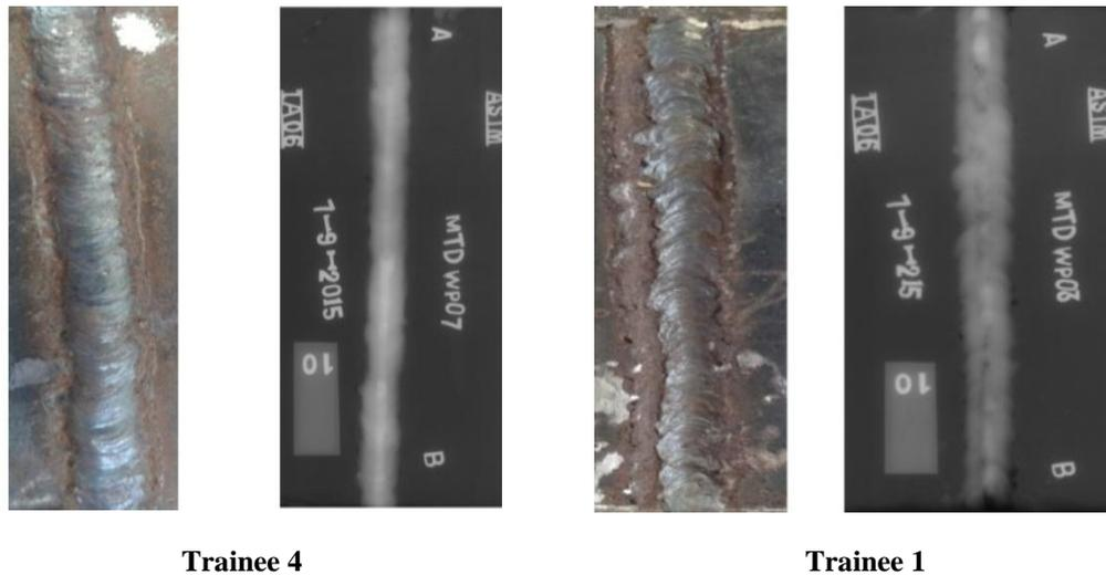
**Fig. 4.5: Bead images of weld pad and corresponding radiograph image (arranged in decreasing order of their quality).**
