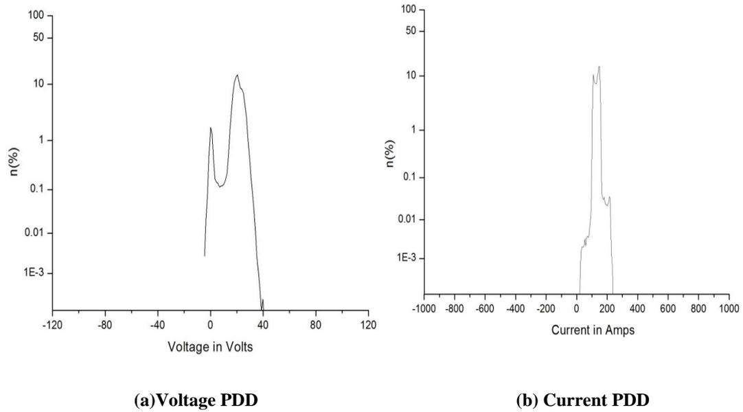
**Fig. 3.9** PDD analysis of the voltage and current data acquired using DSO.
