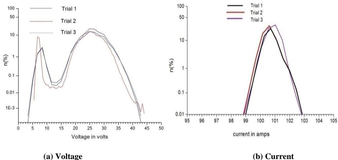
**Fig. 4.19: PDD analysis of voltage and current for E 7018 electrode and inverter power supply.**
