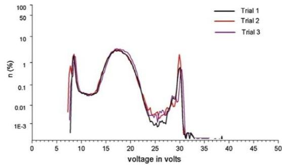
Fig. 3: PDD using E6010 electrode
