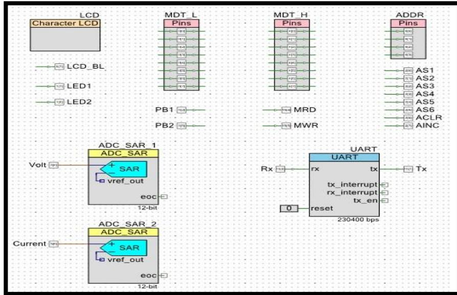
Fig.5.7: Top schematic of PSoC-5 based design.
