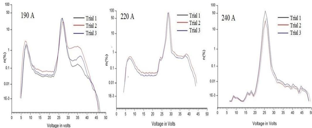
**Fig. 4.37: Voltage and current PDD of GMAW process with 100% Ar.**
