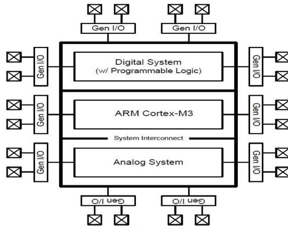
**Fig. 2.13: PSoC-5 LP block diagram [66].**
