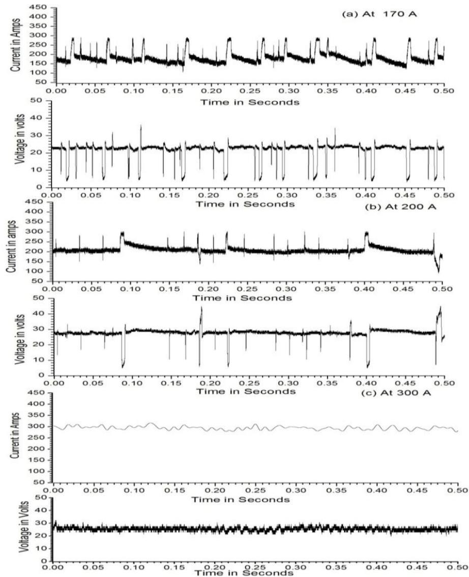
**Fig. 4.31:** Voltage and current oscillogram of GMAW process with 80 % Ar and 20 % CO<sub>2</sub>.
