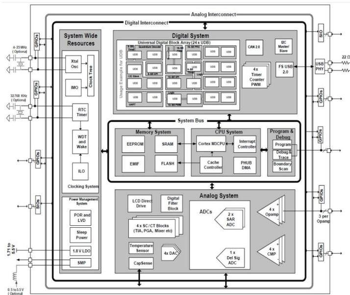
Fig. 2.11: PSoC 5 architecture [59] (LCD- Liquid crystal display, OpAmp-Operational Amplifier, RTC –Real time control, SRAM-Static Random Access Memory, XTAL Osc- External Oscillator, EEPROM- Electrically Erasable Programmable Read-Only Memory).
