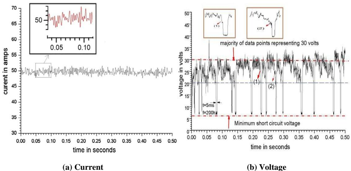
**Fig. 4.16: Voltage and current signature pattern using E 6010 electrode and inverter power supply.**
