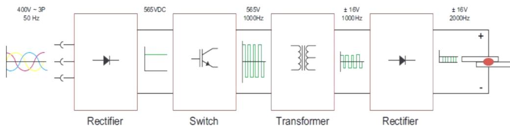
**Fig. 2.6: Block diagram for inverter technology.**
