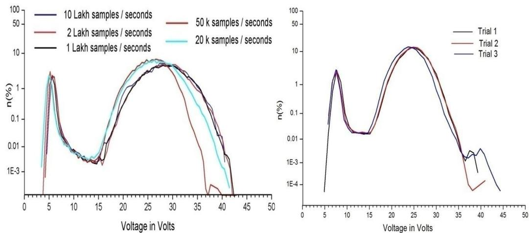
(a) PDD with varying acquisition rates. (b) Three trials of PDD at 100,000 samples/s.
