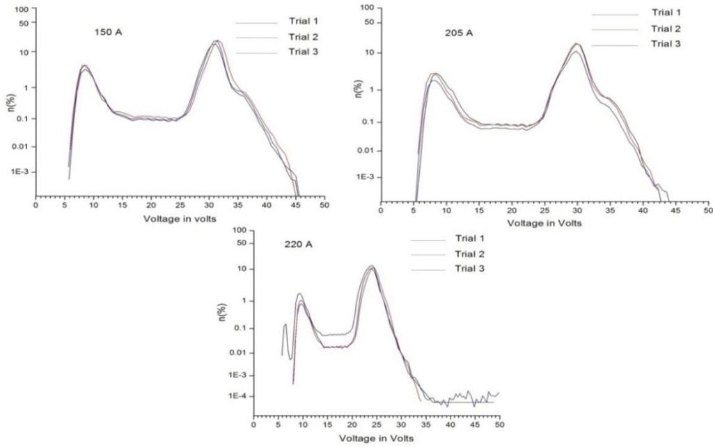
**Fig. 4.35: Voltage and current PDD of GMAW process with 100 %CO<sub>2</sub>.**
