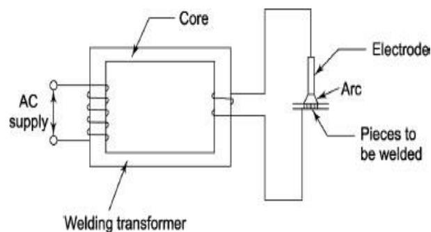
**Fig. 2.5: Welding transformer.**
