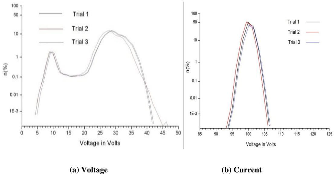
Fig. 4.20: PDD analysis of voltage and current for E 6013 electrode using inverter power supply.
