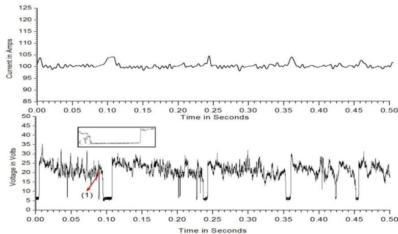
**Fig. 4.18: Voltage and current signature pattern using E 6013 electrode and inverter power supply.**
