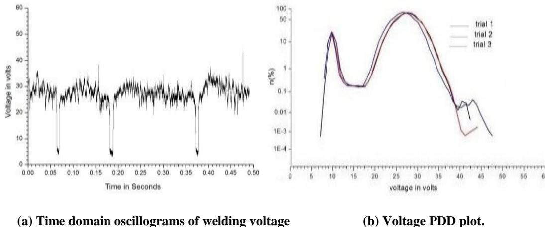
(a) Time domain oscillograms of welding voltage
