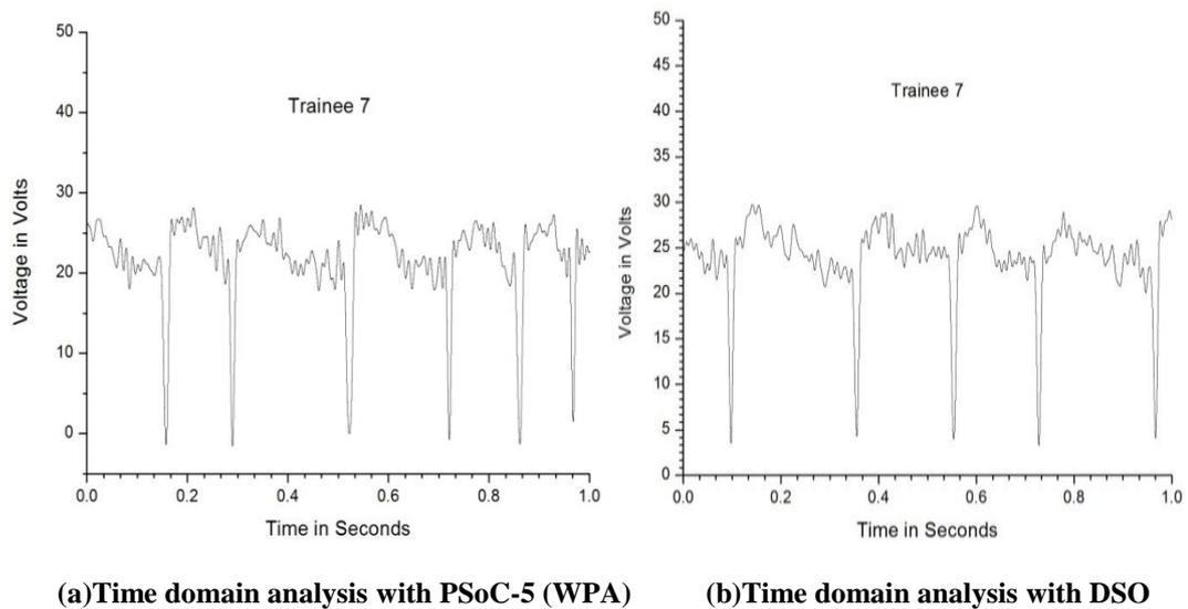
**Fig. 5.19: Time domain analysis of the voltage data acquired using PSoC-5 (WPA) and DSO.**
