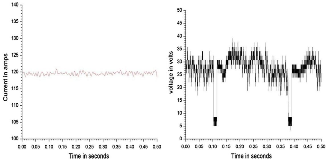
**Fig. 4.29: Voltage and current oscillogram obtained during welding using unbaked E 7018 electrode.**
