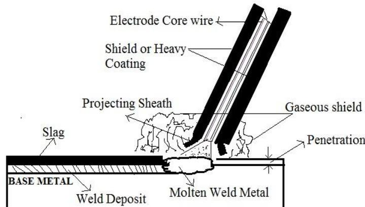
**Fig. 2.1: Shielded metal arc welding.**
