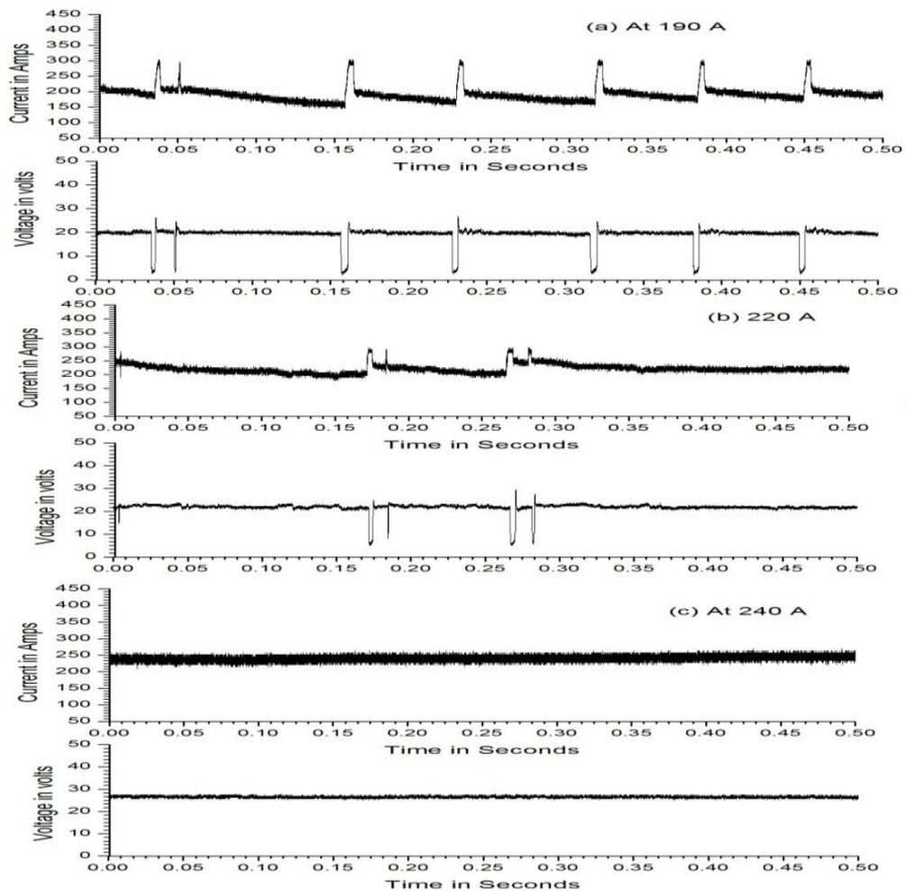
**Fig. 4.36: Voltage and current oscillogram of GMAW process with 100% Ar.**
