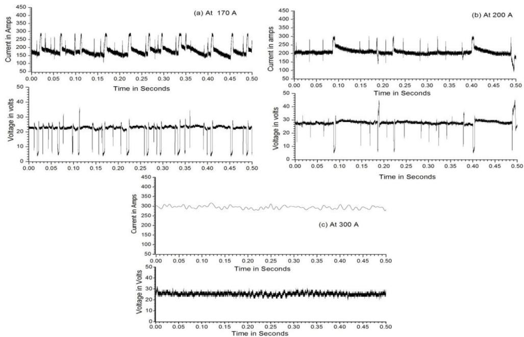
Fig. 5: Current and voltage oscillogram of GMAW welding using 80% Ar & 20% CO<sub>2</sub>.
