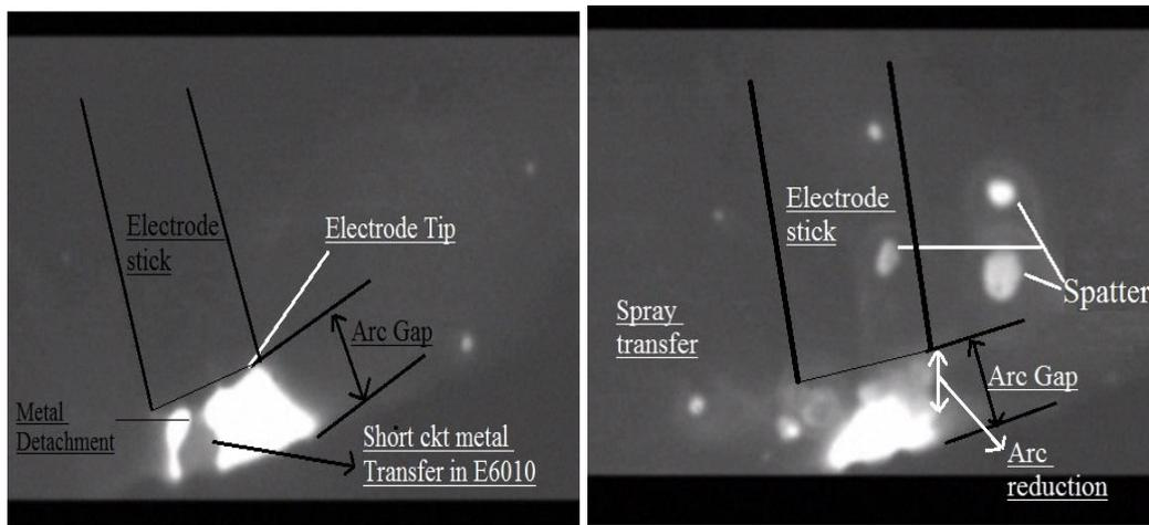
**(a) Short circuit and (b) Spray mode of metal transfer image obtained using high speed camera**
