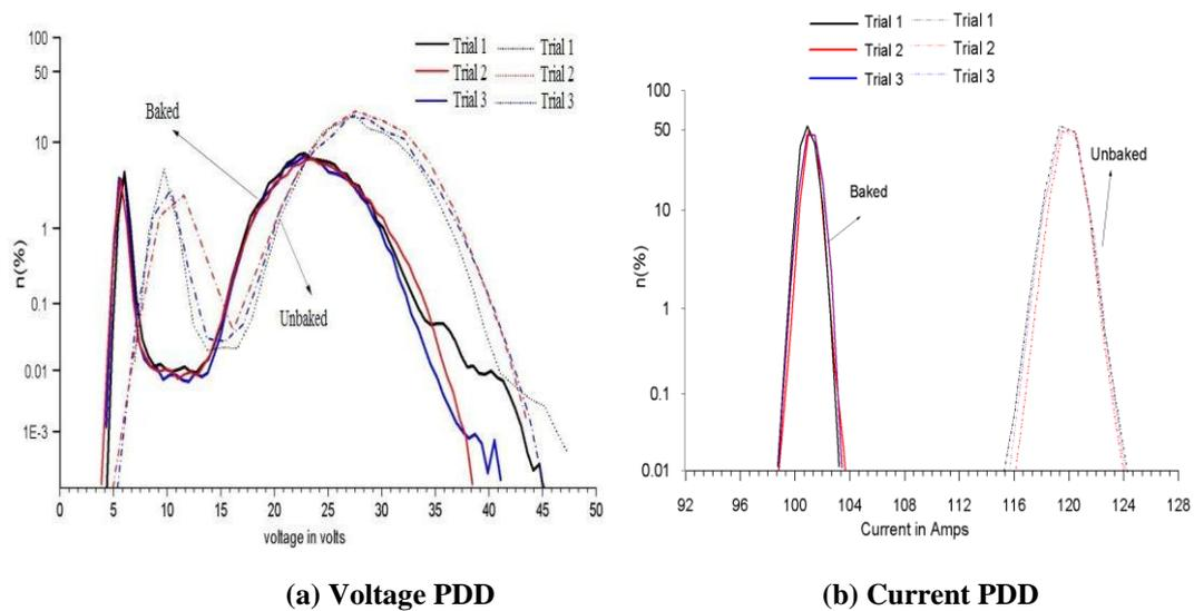
**Fig. 4.30: PDD analysis of voltage and current characteristic behavior of unbaked and baked electrode.**
