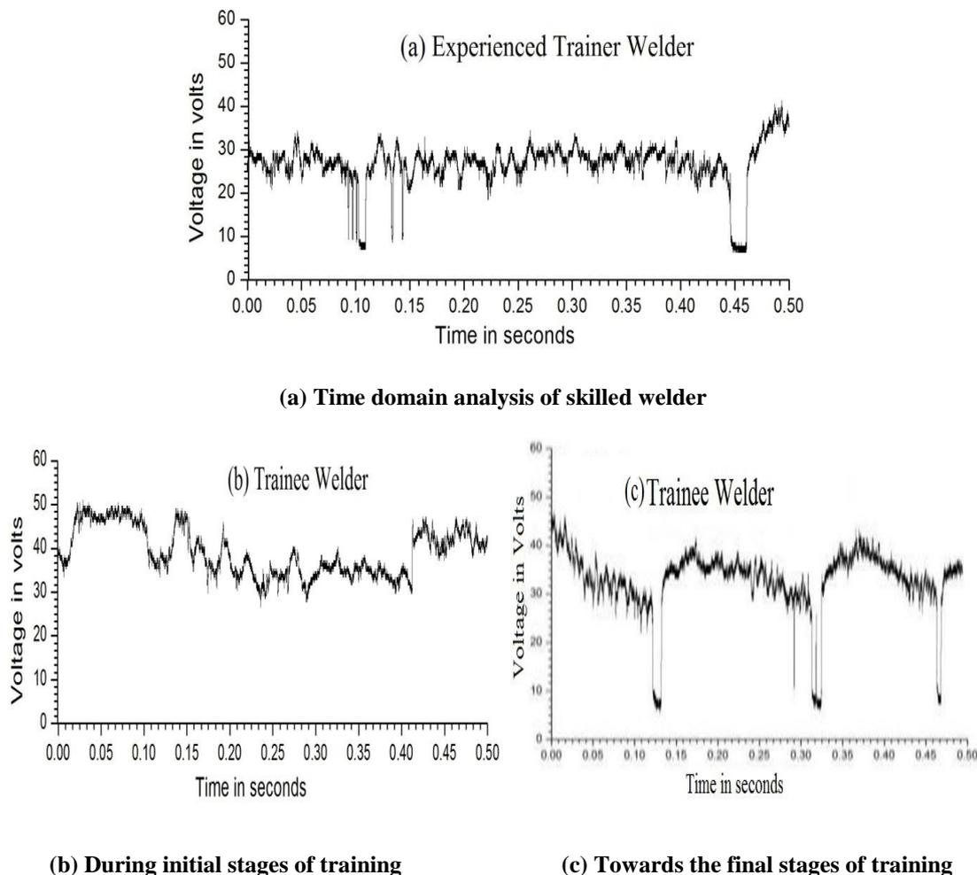
**Fig. 4.3: Time domain analysis of Skilled (Trainer) and less skilled (Trainee) welder.**
