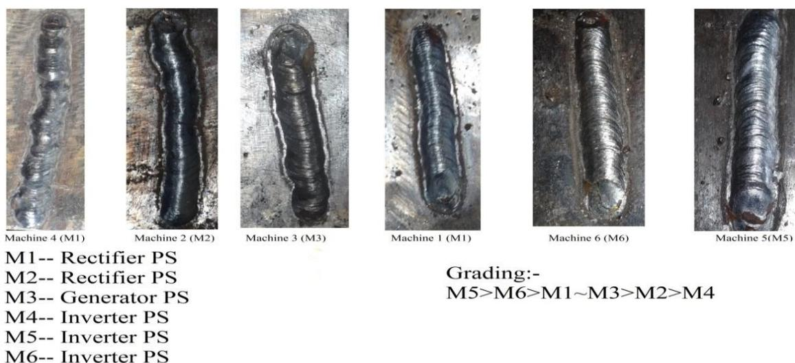
**Fig. 4.14:** Weld beads obtained by welding from various power sources.
