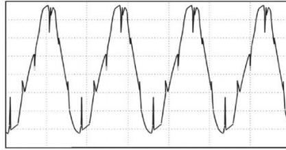
**Fig. 2.14: Waveform distorted by notching [67].**
