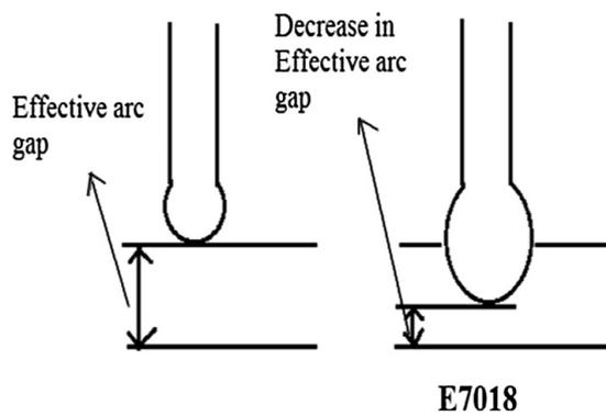
Fig. 4.22: Schematic of short circuit metal transfer in E 7018 and E 6013 electrodes.
