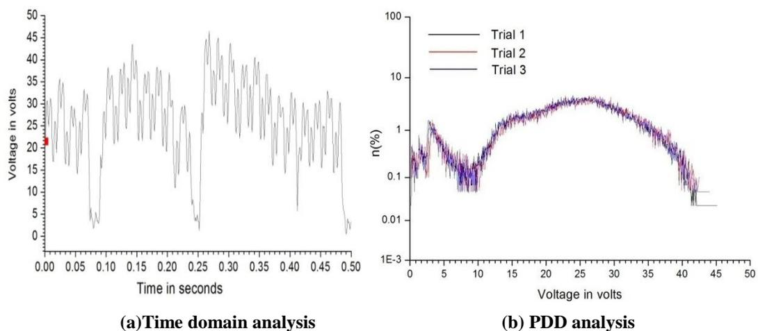
**Fig. 5.4:** Time domain and PDD analysis of the voltage data acquired using PSoC-3 design.
