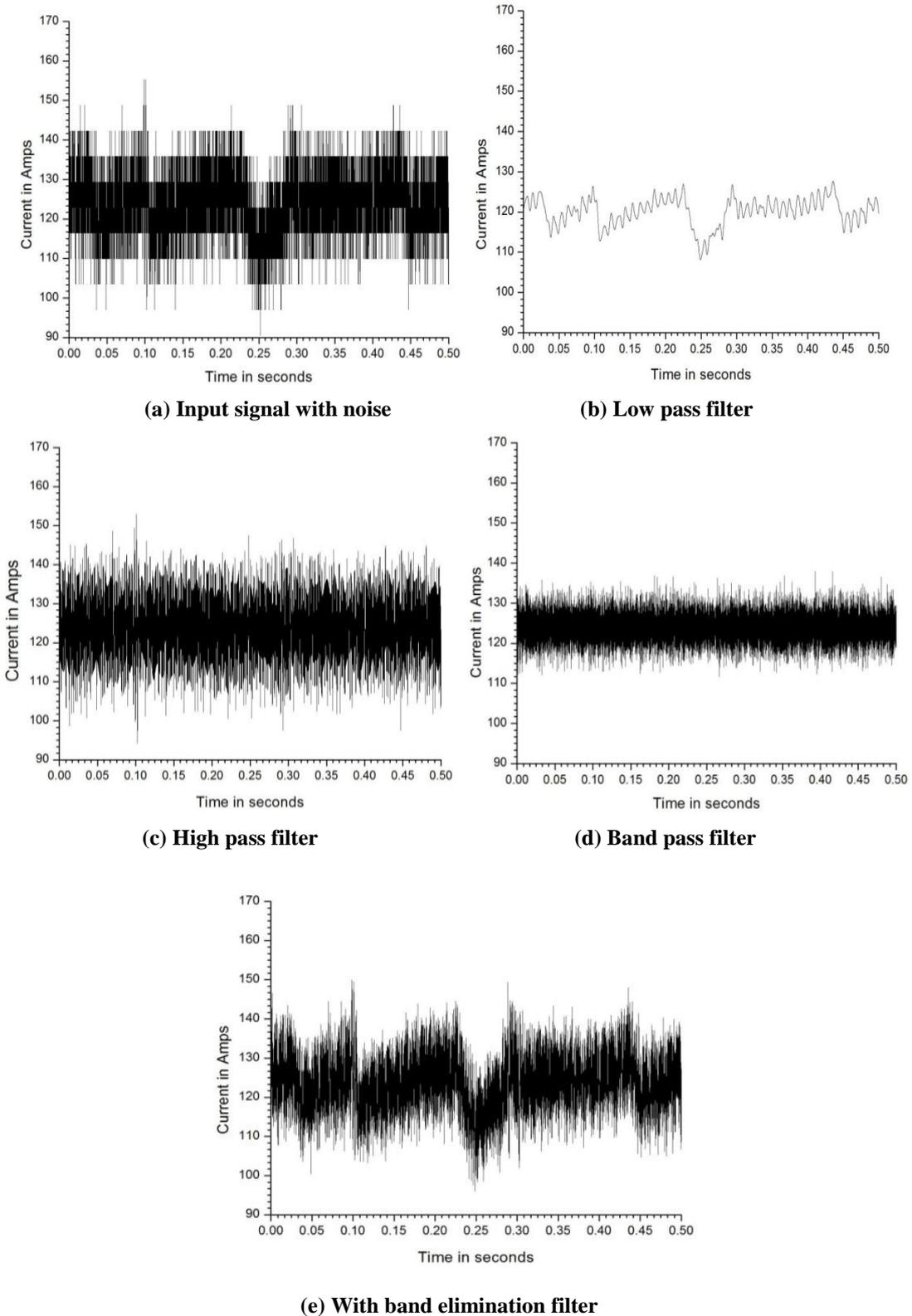
**Fig. 3.4:** Samples of filtered welding current with various filtering techniques (a) shows input signal with noise, (b) filtered input with low pass filter, (c) with high pass filter, (d) with band pass filter, (e) with band elimination filter.
