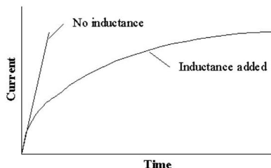
**Fig. 2.4 Effect of inductance on welding current.**
