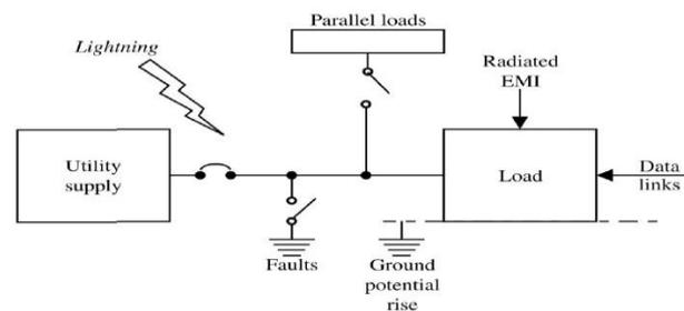
**Fig. 2.15: Noise emanating from electrical systems within a facility [67].**
