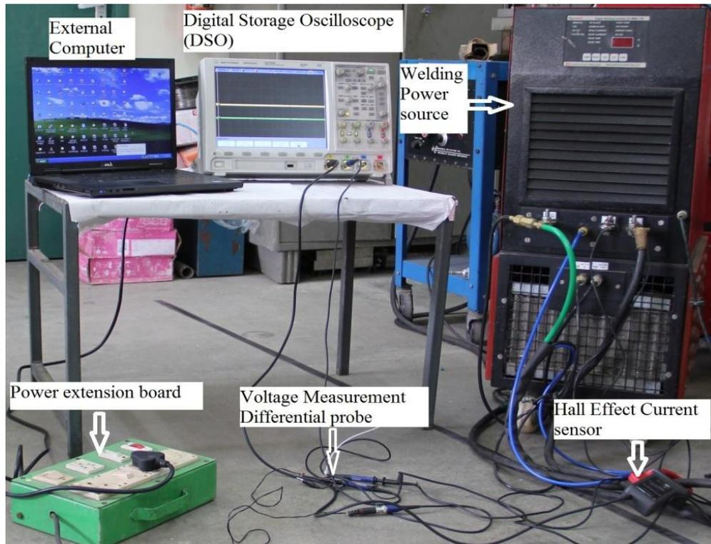
**Fig. 3.2: Photograph of welding setup with data acquisition unit.**
