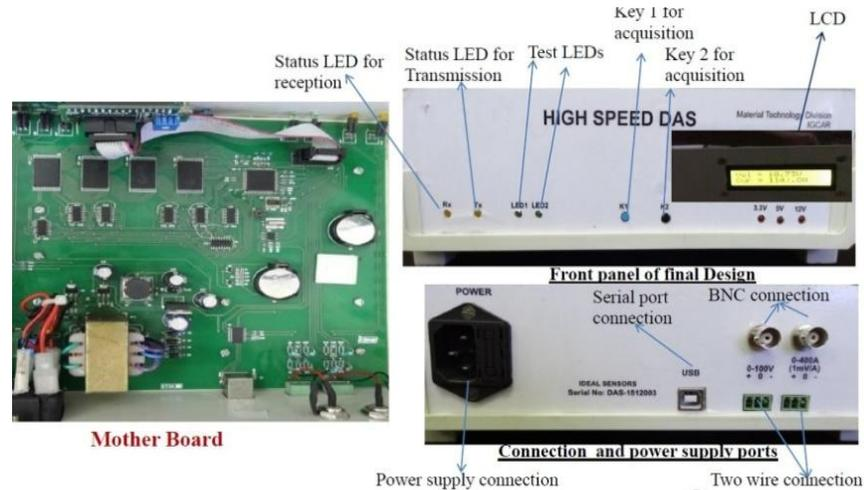
**Fig. 6: Mother board with front and back panel of final WPA.**
