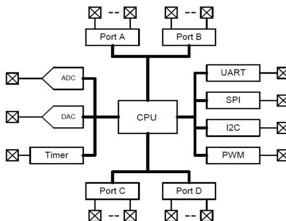
**Fig. 2.12: Block diagram of typical MCU [66] (DAC-Digital to Analog Converter, SPI-Serial Port Interface, PWM-Pulse Width Modulation).**
