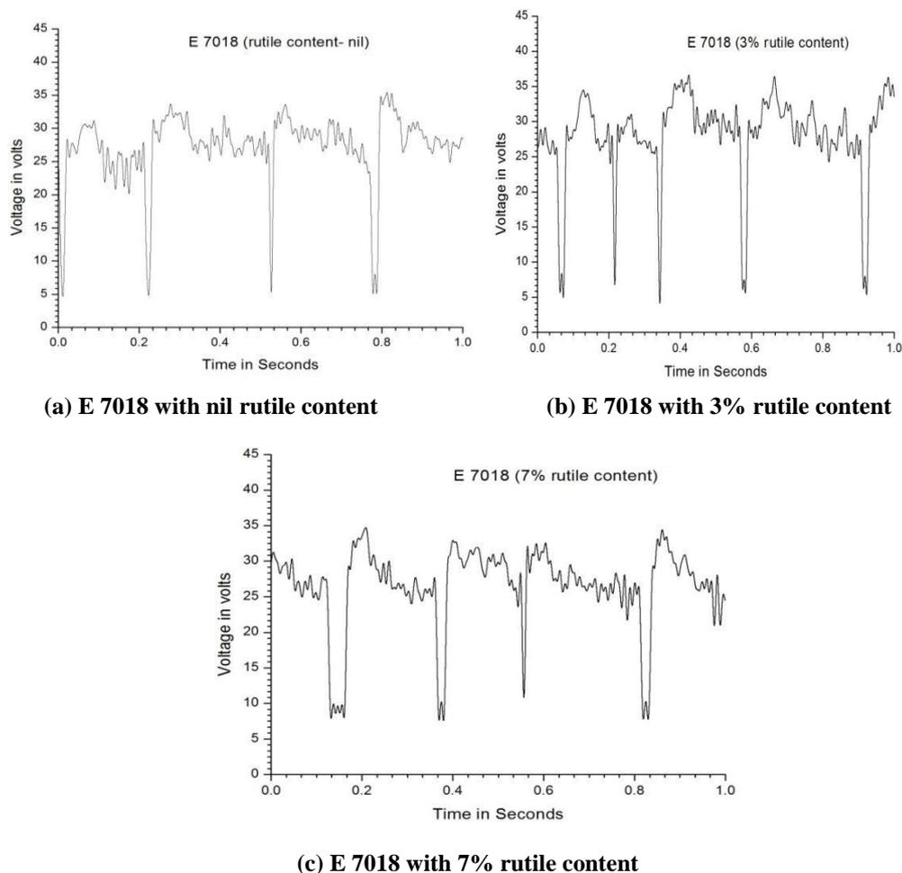
**Fig. 4.27: Time domain analysis of E 7018 electrode with different rutile compositions.**
