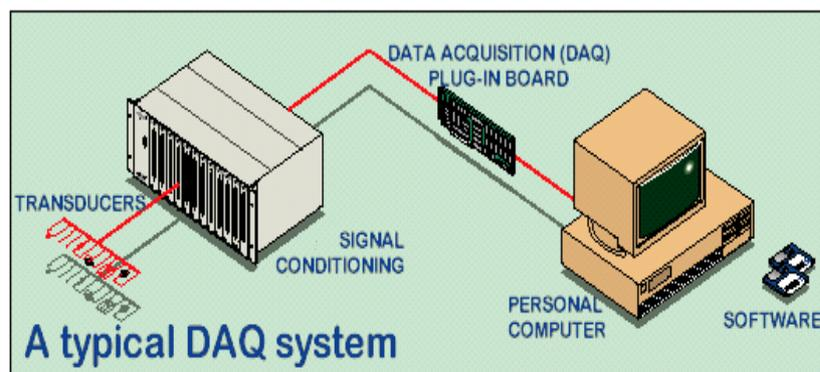
**Fig. 2.8:** Various stages in a DAS [55].
