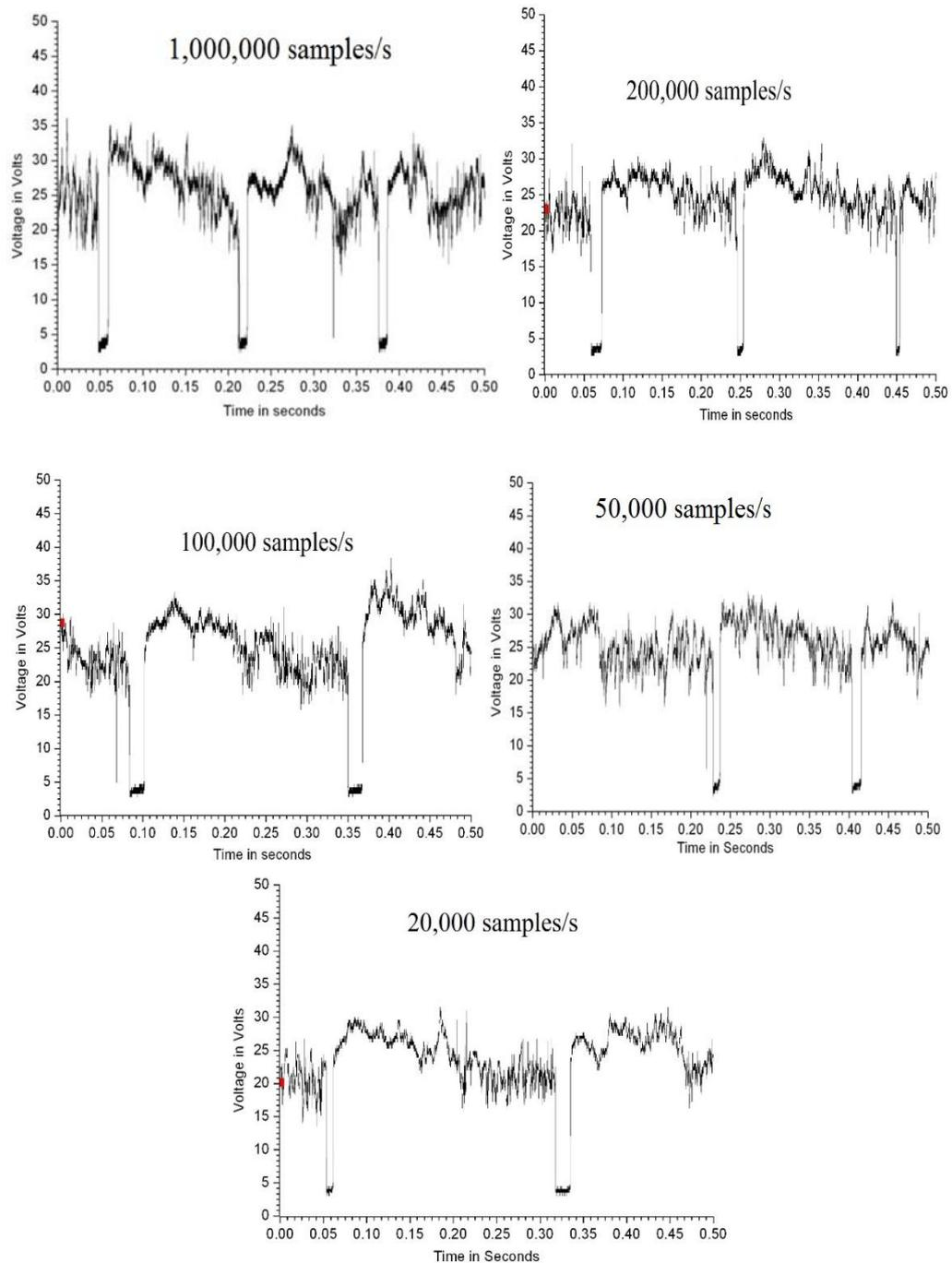
**Fig. 3.7: Time domain analysis of welding voltage acquired at different acquisition rates.**
