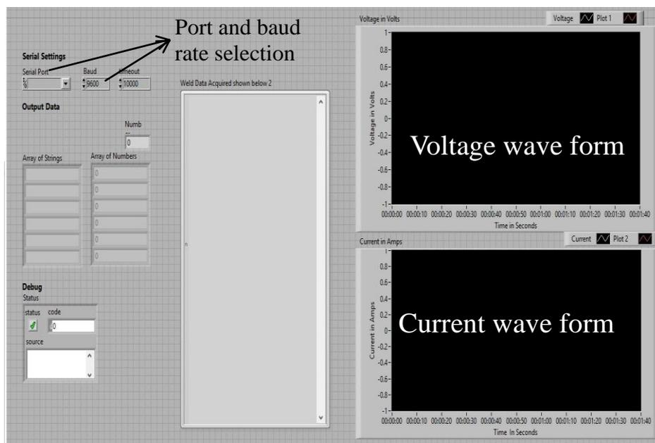
**Fig. 5.12: Real time visualization/analysis of current and voltage signal with lab view.**
