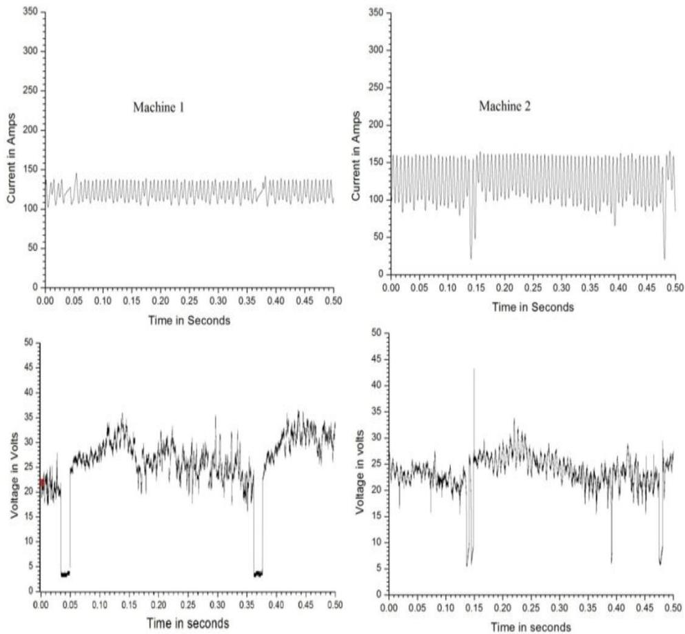
**Fig. 4.10: Time domain analysis of voltage and current data obtained from different rectifier power sources.**
