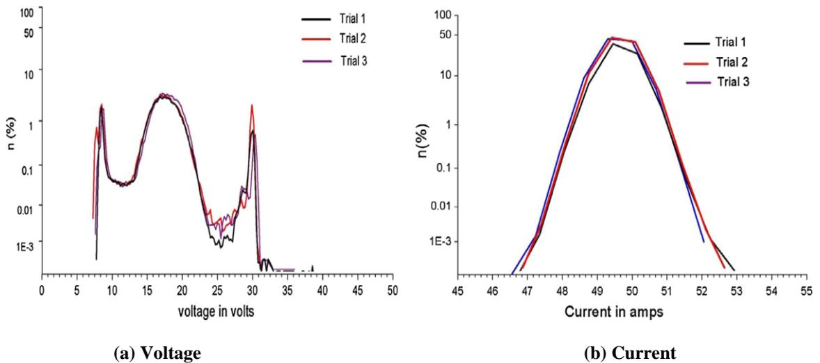
**Fig. 4.23: Voltage and current PDD for E 6010 electrode using inverter power supply.**
