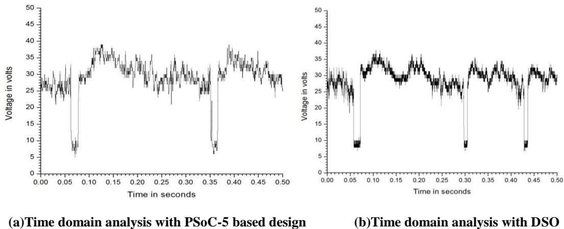
**Fig. 5.17:** Time domain analysis of the voltage data acquired using PSoC-5 (WPA) and DSO.
