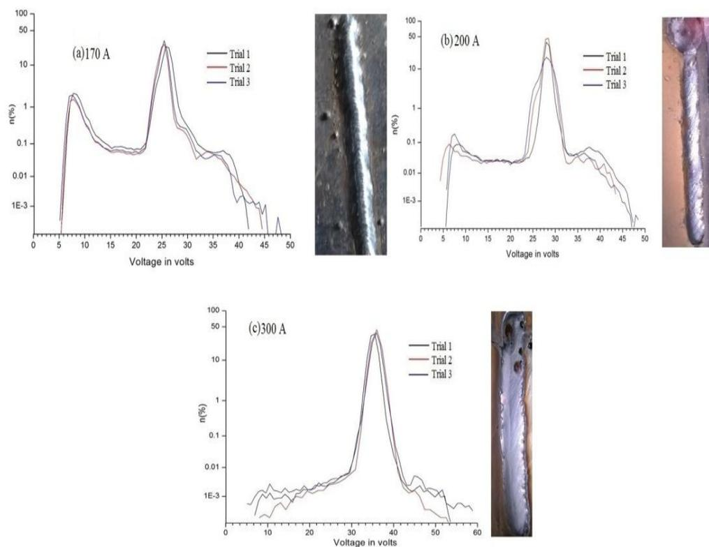
**Fig. 4.32: Voltage, current PDD and corresponding bead Image of GMAW process for different values of current for a combination of 80 % Ar and 20 % CO<sub>2</sub>.**
