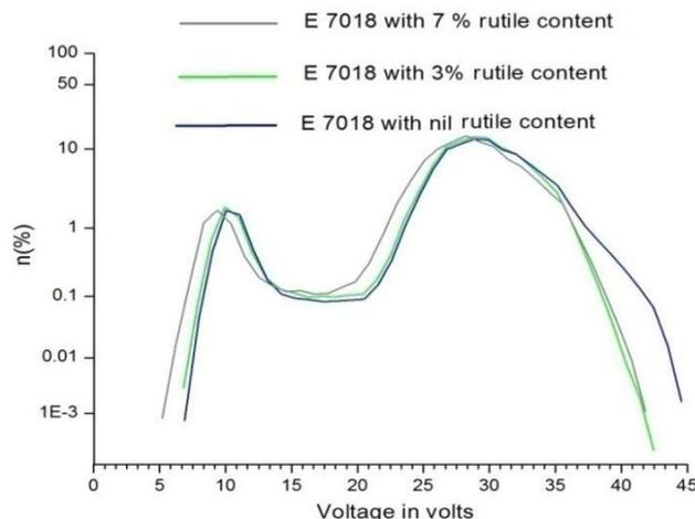
**Fig. 4.28: PDD analysis of E 7018 electrode with varying rutile content.**
