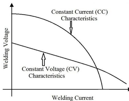
**Fig. 2.3: Characteristic curve for welding power source.**
