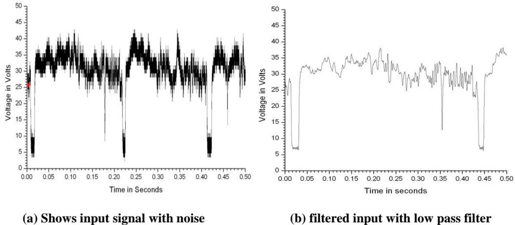
**Fig. 3.6: Samples of filtered welding voltage.**
