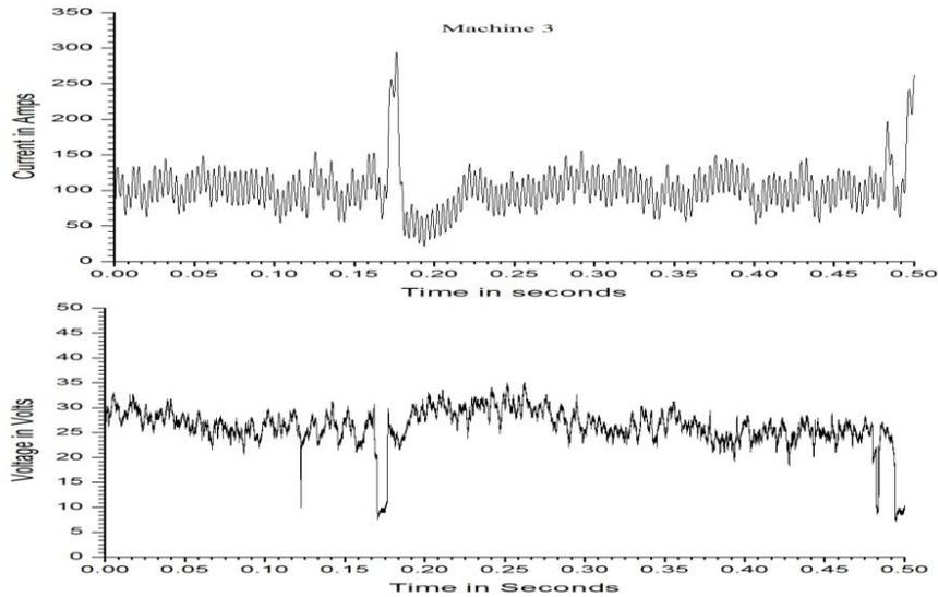
**Fig. 4.11:** Time domain analysis of voltage and current data obtained from a generator power source.
