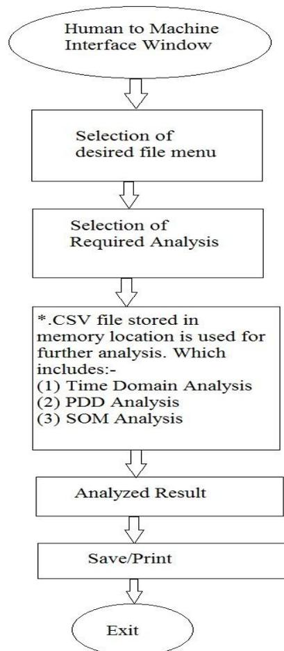
Fig. 5.14: Flow diagram of interface window for analyzing acquired data.
