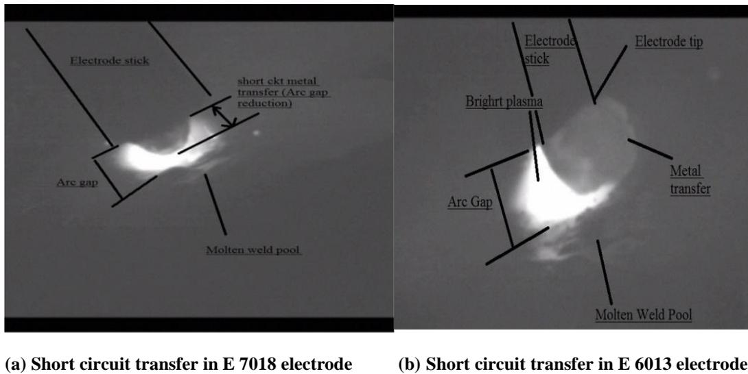
Fig. 4.21: Short circuit image seen with high speed camera.
