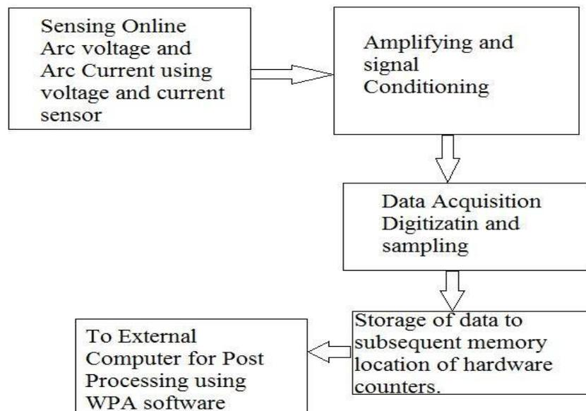
**Fig. 5.9: Working schematic of WPA (PSoC-5 design).**
