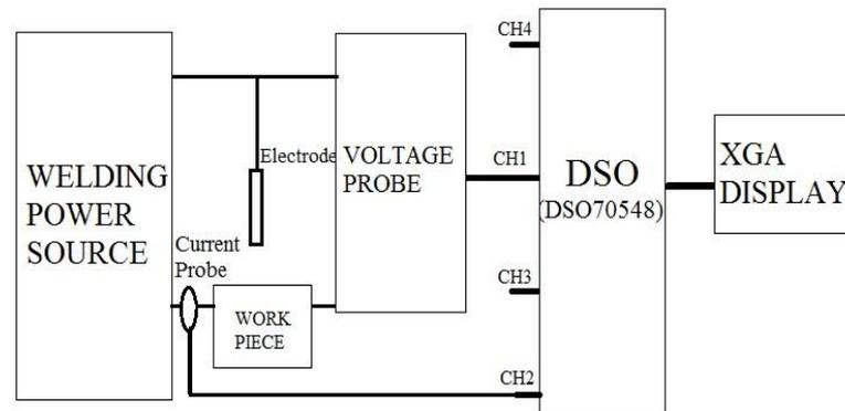
**Fig. 3.1: Block diagram of data acquisition setup.**
