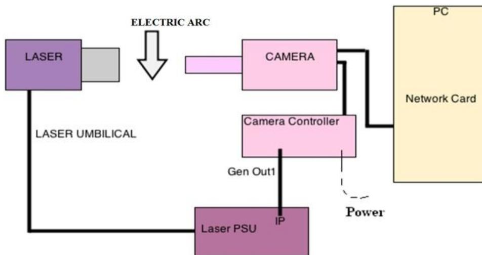
**Fig. 4.15: Schematic of high speed camera assembly.**
