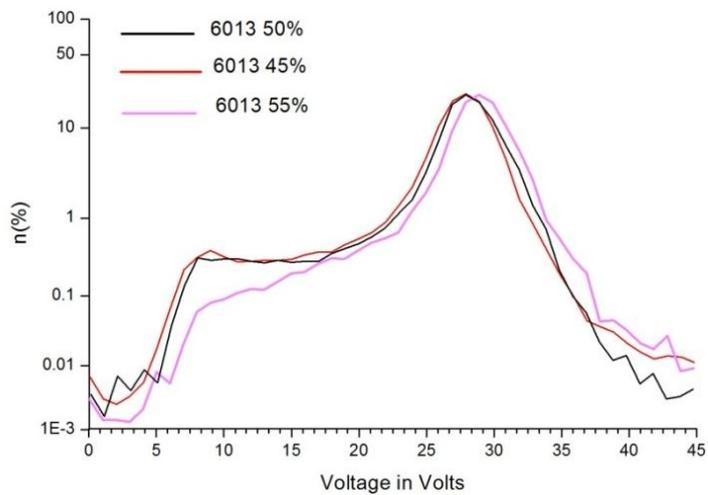
Fig. 5.24: PDD analysis of E 6013 electrode with varying rutile content.
