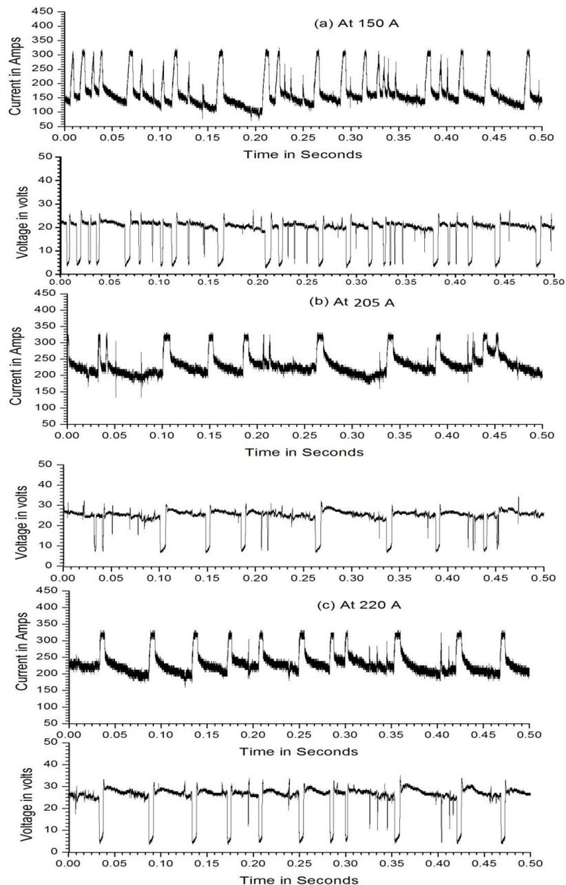
**Fig. 4.34: Voltage and current oscillogram of GMAW process with 100% CO<sub>2</sub>.**
