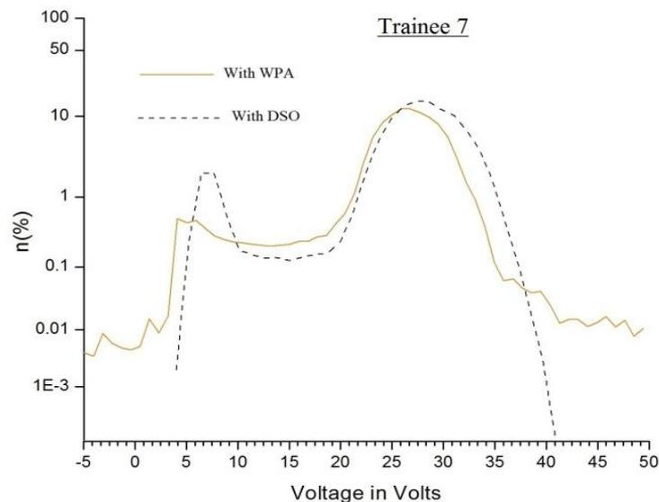
**Fig. 5.20: PDDs obtained with the data acquired by DSO and WPA for one typical trainee welder.**
