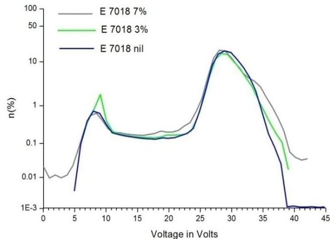
**Fig. 5.26: PDD analysis of E 7018 electrode with varying rutile content.**
