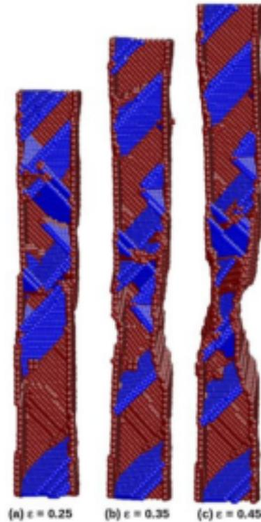
Figure 4.8: Deformation behaviour in small size  $\langle 100 \rangle$  Cu nanowires with cross section width  $(d) = 3.615$  nm under tensile loading. The deformation occurring by slip of partial dislocations can be seen at all strains. The blue color atoms represent the stacking faults and the red color atoms indicate the surfaces and dislocation core. The perfect FCC atoms were removed for clarity.
