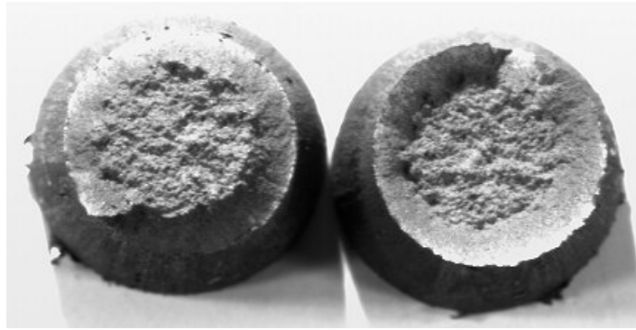
Fig. 2.15: Typical cup-cone fracture appearance of un-notched tensile specimen [32]
