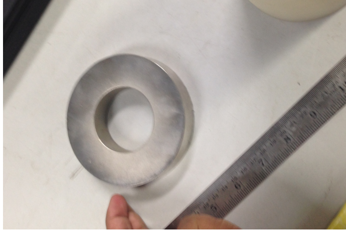
Figure 4.5: Permanent Ring magnet for providing axial field inside the plasma source.
