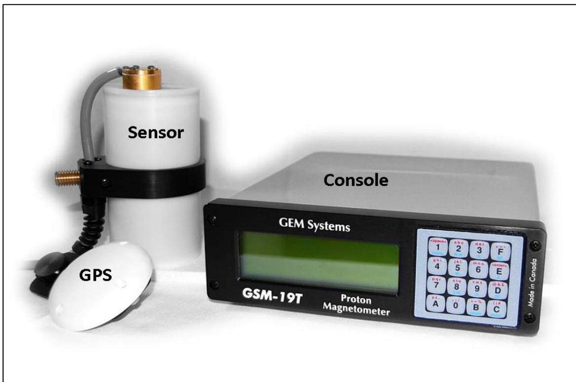
Figure 3.1 GEM Systems, GSM 19T Proton Precision Magnetometer used for Data Acquisition in the survey area ([www.gemsys.ca](http://www.gemsys.ca))
