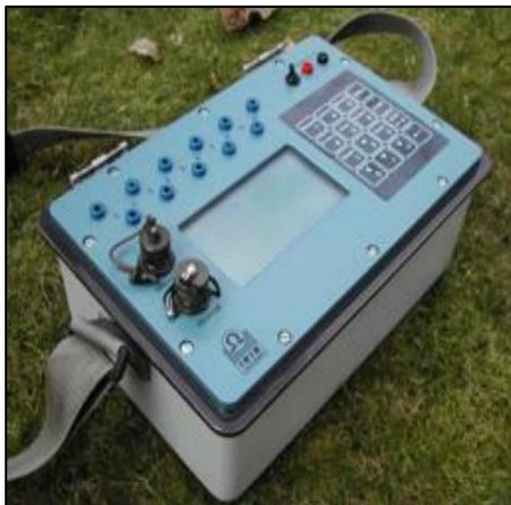
Figure 4.5 Multi electrode IRIS IP Receiver
