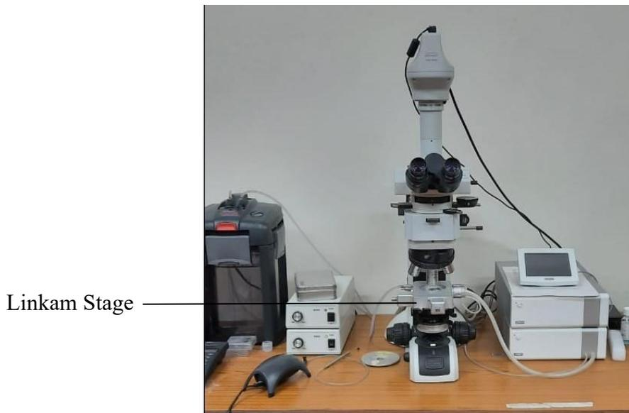
Figure 5.16 Nikon petrological microscope mounted with Linkam cooling/freezing stage
