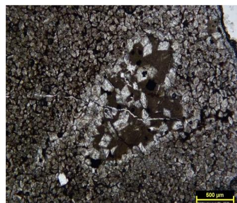
Figure 5.12 Photomicrograph showing cavity filled with coarser dolomite rhombs & micrite in microspar dolomite bearing
