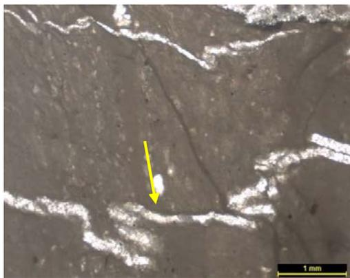
Figure 5.11 Photomicrograph showing calcite filled along microfractures which are interconnected giving a folded appearance in brecciated limestone.
