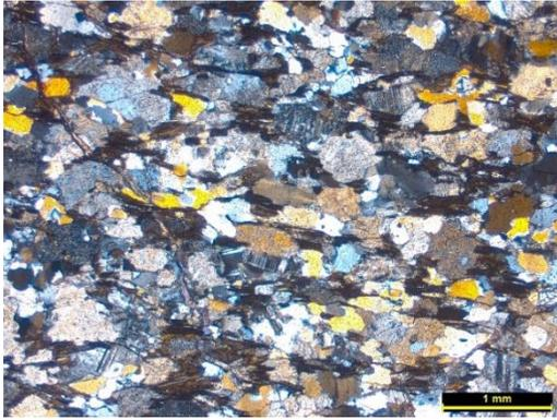
Figure 5.2 Photomicrograph showing crude foliation in basement granite. TL, XN
