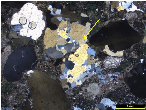
Figure 5.4 Photomicrograph showing crushed granite fragments in brecciated granite TL,XN
