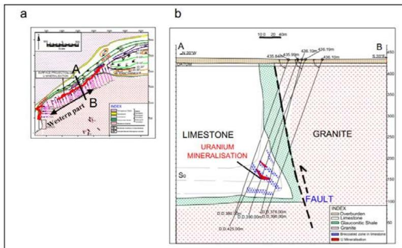
Figure 4.3 (a) Geological map showing location of transverse section line (b) Representative transverse section through boreholes in western part of Kanchankayi area depicting the structure and the uranium mineralisation zones in limestone (after AMD unpublished annual report, 2016)
