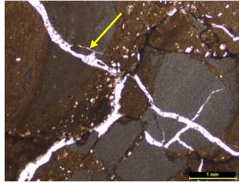
Figure 5.8 Photomicrograph showing sparry calcite veins cutting across the brecciated zones in brecciated limestone. TL, XN
