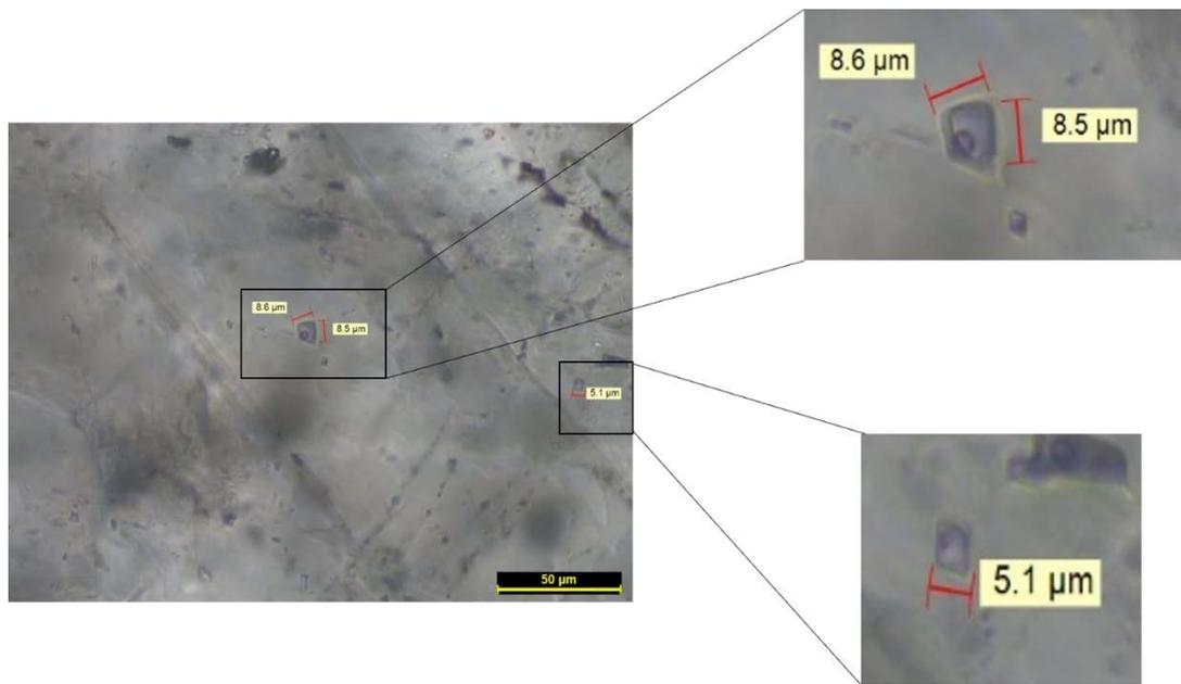
Figure 5.20 Primary inclusions in calcite
