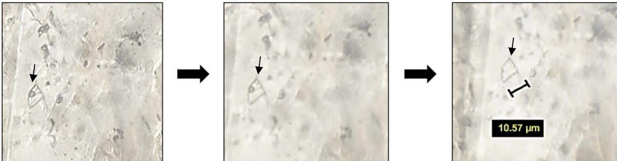
Figure 5.18 Homogenisation of bi-phase (vapour rich) fluid inclusion in calcite with increasing temperature (a) Temp: 40<sup>0</sup>C, degree of fill 80 percent (b) Temp:96<sup>0</sup>C, degree of fill: 85 percent (c) Temperature: 165<sup>0</sup>C, degree of fill 100 percent
