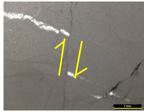
Figure 5.10 Photomicrograph showing offset of thin calcite veins in fractured limestone. TL, 1N
