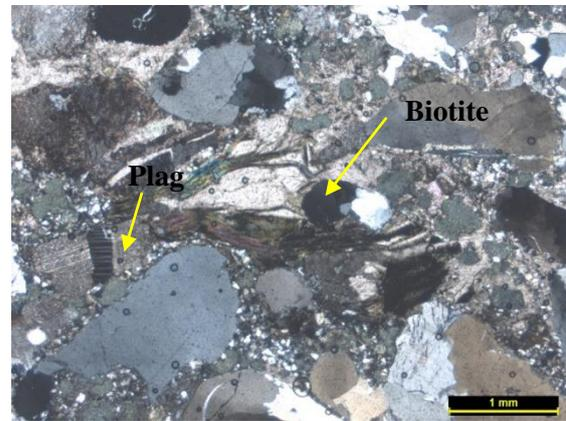
Figure 5.5 Photomicrograph showing deformed biotite and kinked plagioclase in granite. TL, XN
