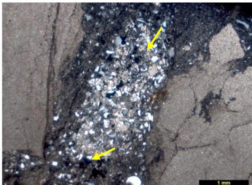
Figure 5.9 Photomicrograph showing small quartz and feldspar fragments in brecciated zones within brecciated limestone. TL, XN
