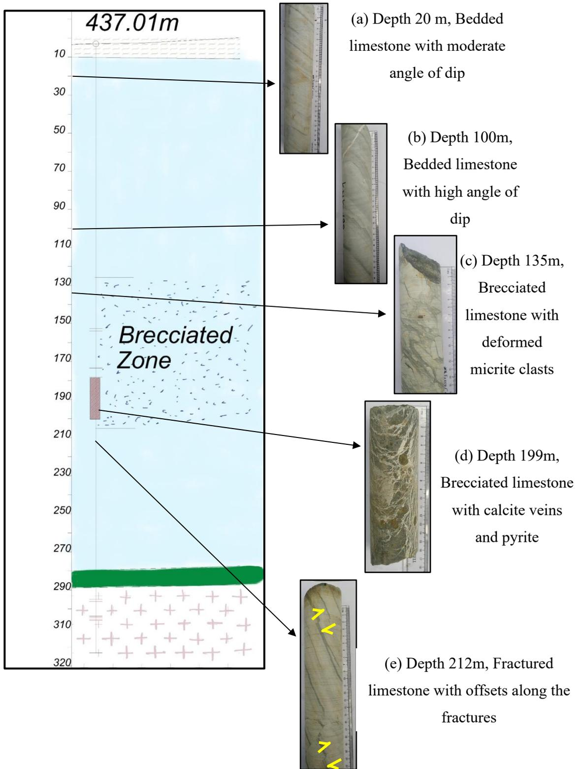
Figure 4.5 Deformation observed along the vertical borehole with increasing depth.
