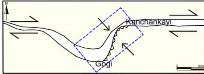
Figure 4.1 Schematic diagram showing development of transpressional zone at restraining bend of dextral slip fault near Gogi-Kanchankayi
