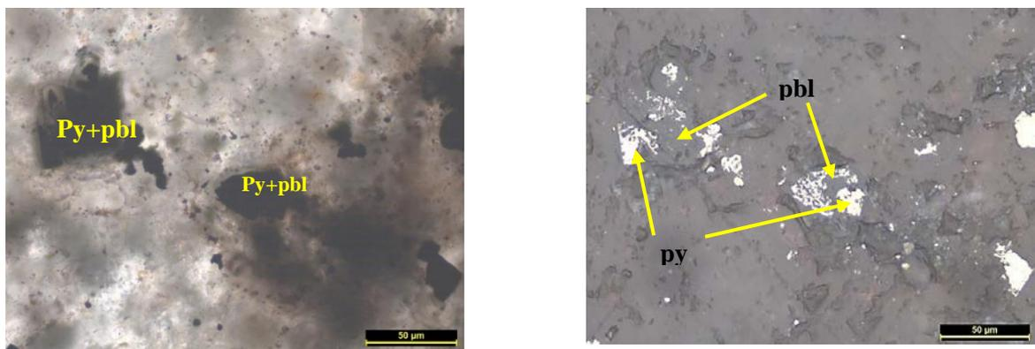
Figure 5.14 Photomicrograph showing pyrite(py) associated with pitchblende(pbl) in brecciated limestone (a) TL, 1N , (b) RL,1N
