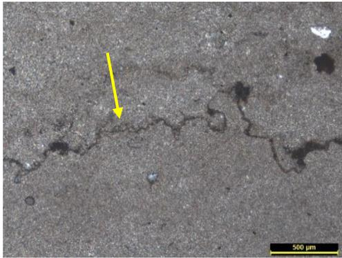
Figure 5.7 Photomicrograph showing stylolites in micritic limestone, TL, 1N
