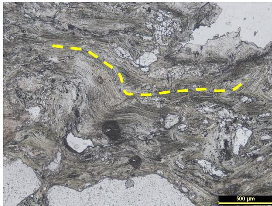
Figure 5.6 Photomicrograph showing deformed altered biotite. TL, 1N
