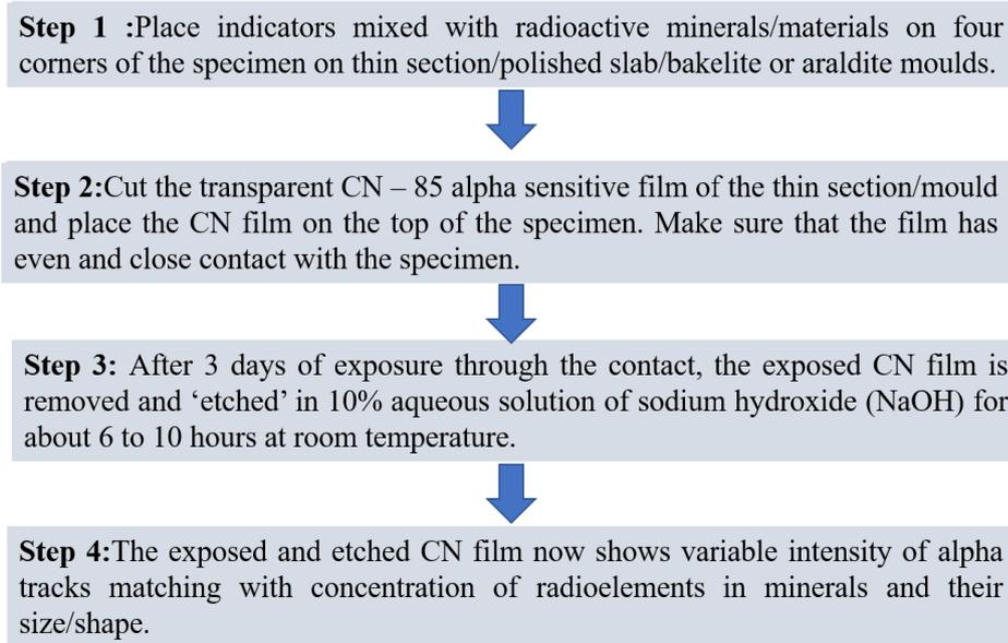
Figure. 5.1 Flowchart of CN Film test
