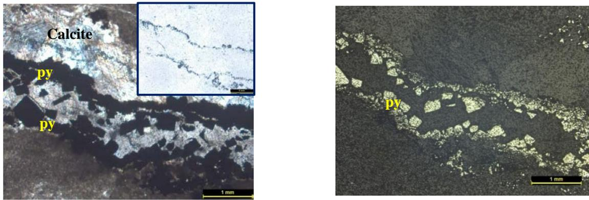
Figure 5.13 Photomicrograph showing pyrite (py) associated with sparry calcite vein, where fine pitchblende(pbl) is surrounding the pyrite grains in brecciated limestone,(a) TL,1N, inset: alpha tracks on CN film (b) RL, 1N
