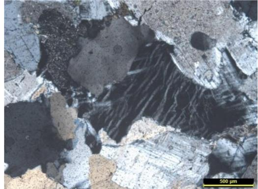
Figure 5.3 Photomicrograph showing perthitic texture in granite, TL, XN
