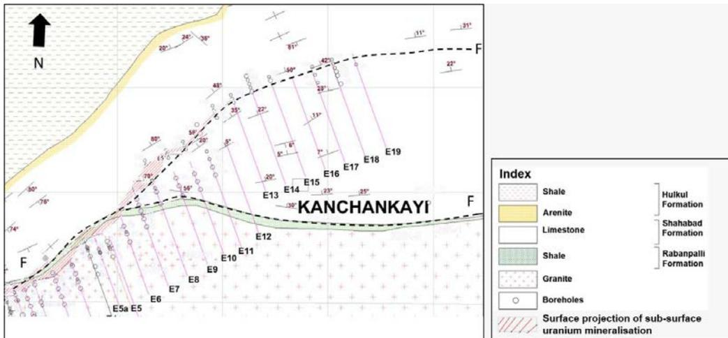
Figure 4.2 Schematic diagram of borehole plan of Kanchankayi sector showing splayed arms of the fault and surface projection of sub-surface uranium mineralisation
