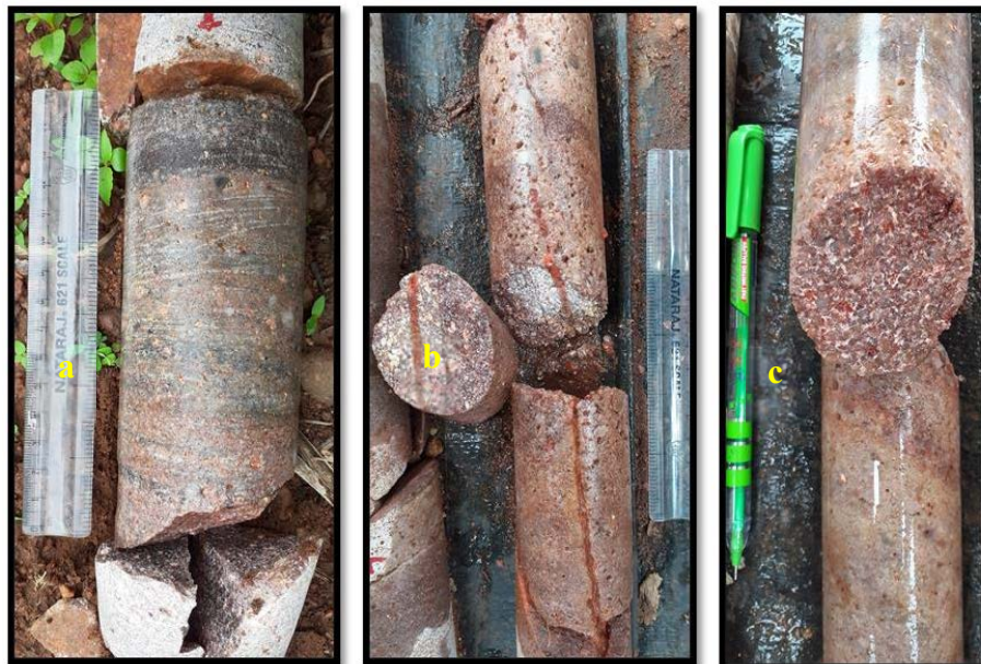
Figure 3.5 Feldspathic arenite; a) cross-stratification, b) ferruginisation along fracture plane c) gritty feldspar and quartz grains.
