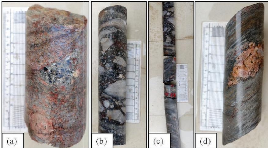
Figure 3.11 (a) Gritty feldspathic quartzite of Rajgarh Formation, (b) Meta-conglomerate composed of pebbles/cobbles of quartz embedded in matrix of quartz, feldspar, tourmaline, magnetite, sericite/muscovite (c) Contact between met-conglomerate and quartz-biotite-sericite schist, (d) Lensoidal quartzo-feldspathic material within quartz-biotite-sericite schist.
