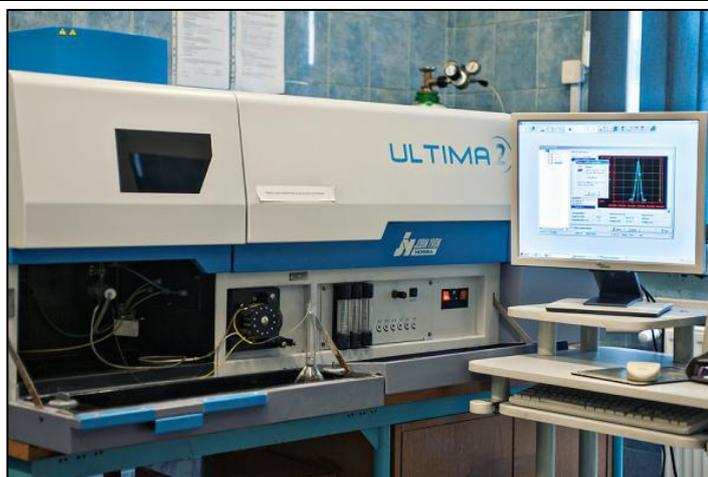
Figure 2.1 Ultima 2 inductively coupled plasma optical emission spectrometer
