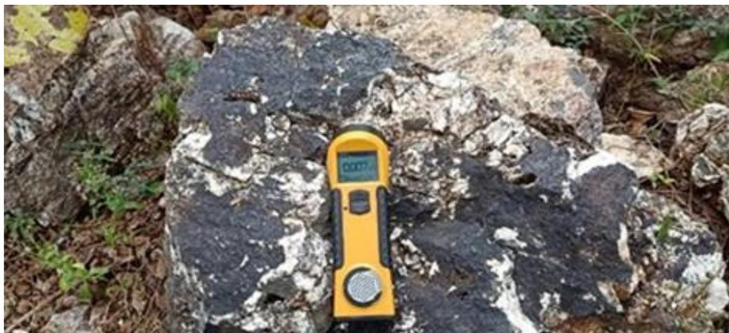
Figure 4.1 Kappa meter for magnetic susceptibility measurements in the field.
