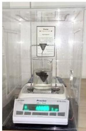
Figure 3.1 Laboratory measurements of density( $\rho$ ).
