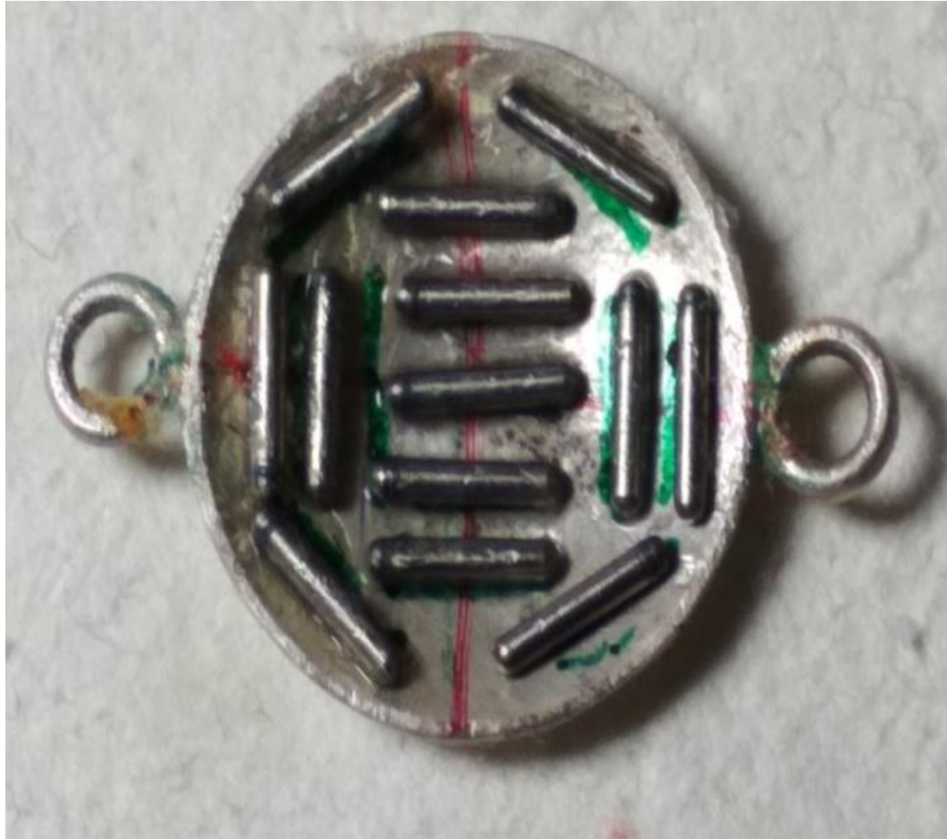
Figure 5.4. A 14 mm diameter silver plaque embedded with 13 ^{125}\text{I} OcuProsta sources. S_K of each seed is 2.94 U.
