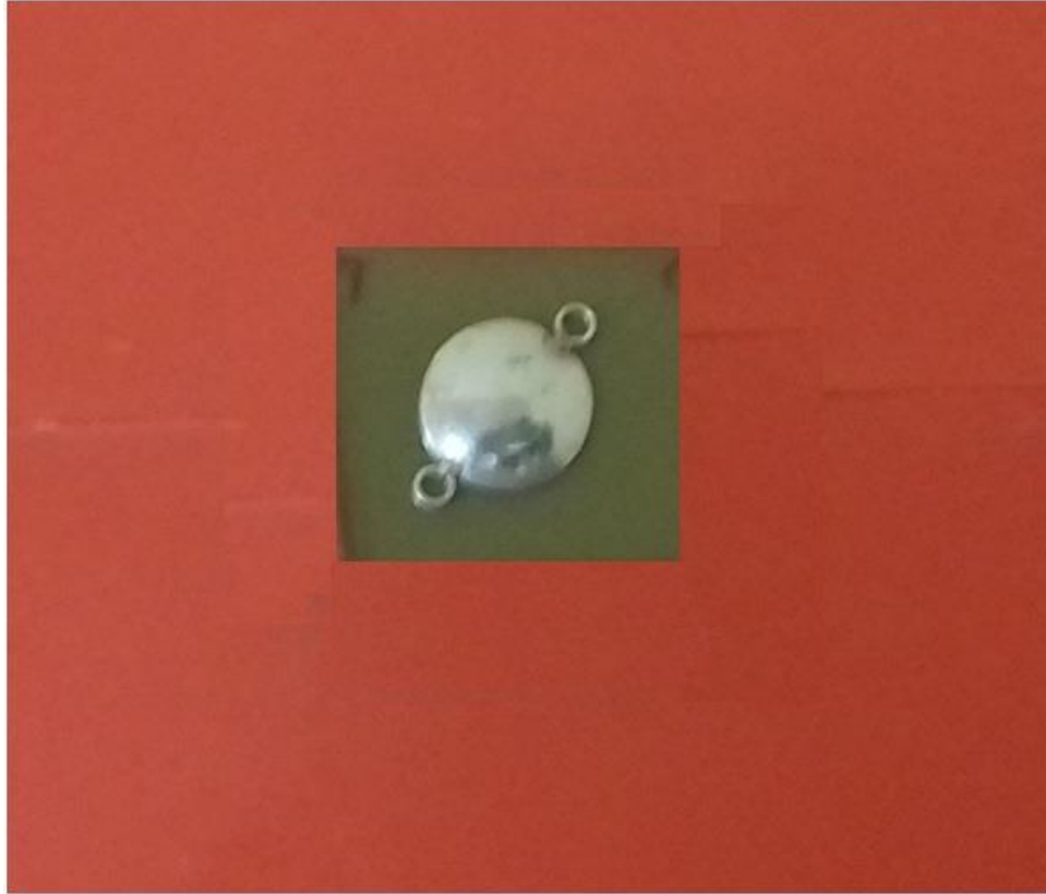
Figure 5.5. 14 mm diameter silver plaque embedded with 13 ^{125}\text{I} OcuProsta seeds, placed over EBT3 Gafchromic film. Films are in the centre of wax phantom. S_k of each seed is 2.94 U.
