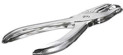
Figure 5. 6mm steel punch plier used for excision of DBS
