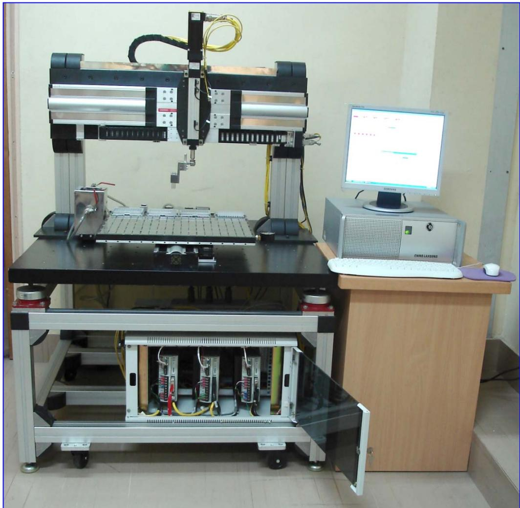
**Figure 2.5** Micro-arraying robotic machine used for preparation of WDDM
