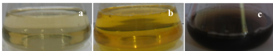
Fig. 3.5.4 Colour of filtrate (a) before addition of chloroplatinic acid (b) after addition of chloroplatinic acid and (c) after formation of platinum nanoparticles
