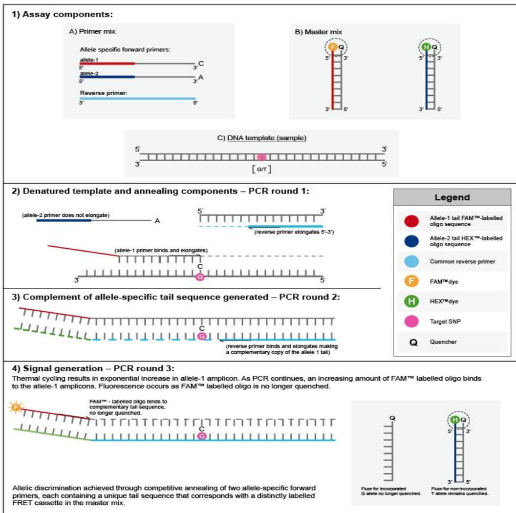
**Fig2.3.4:** Schematic drawing of KASP chemistry. (Source: <http://www.kbioscience.co.uk>)
