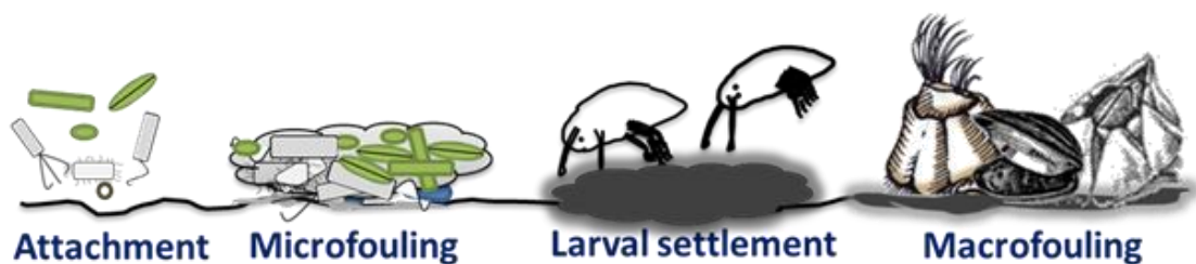
Fig. 1.3. Steps in macrofouling development on submerged surfaces (Adapted from [69]).
