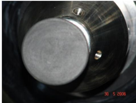
FIG. 3.6 A planar graphite cathode.
