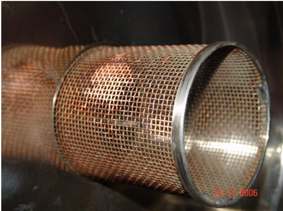
FIG. 3.13 Coaxial vircator copper anode mesh.
