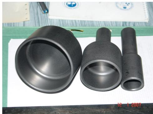
FIG. 3.8 Annular graphite cathodes of various diameters.
