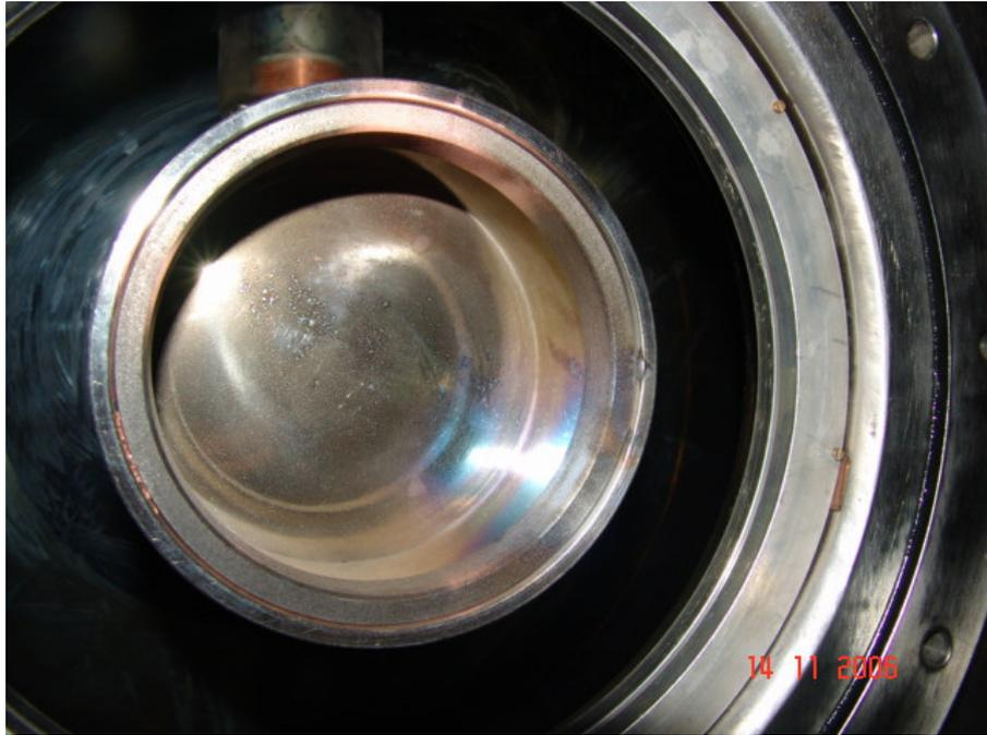
FIG. 3.12 Coaxial vircator graphite annular cathode.
