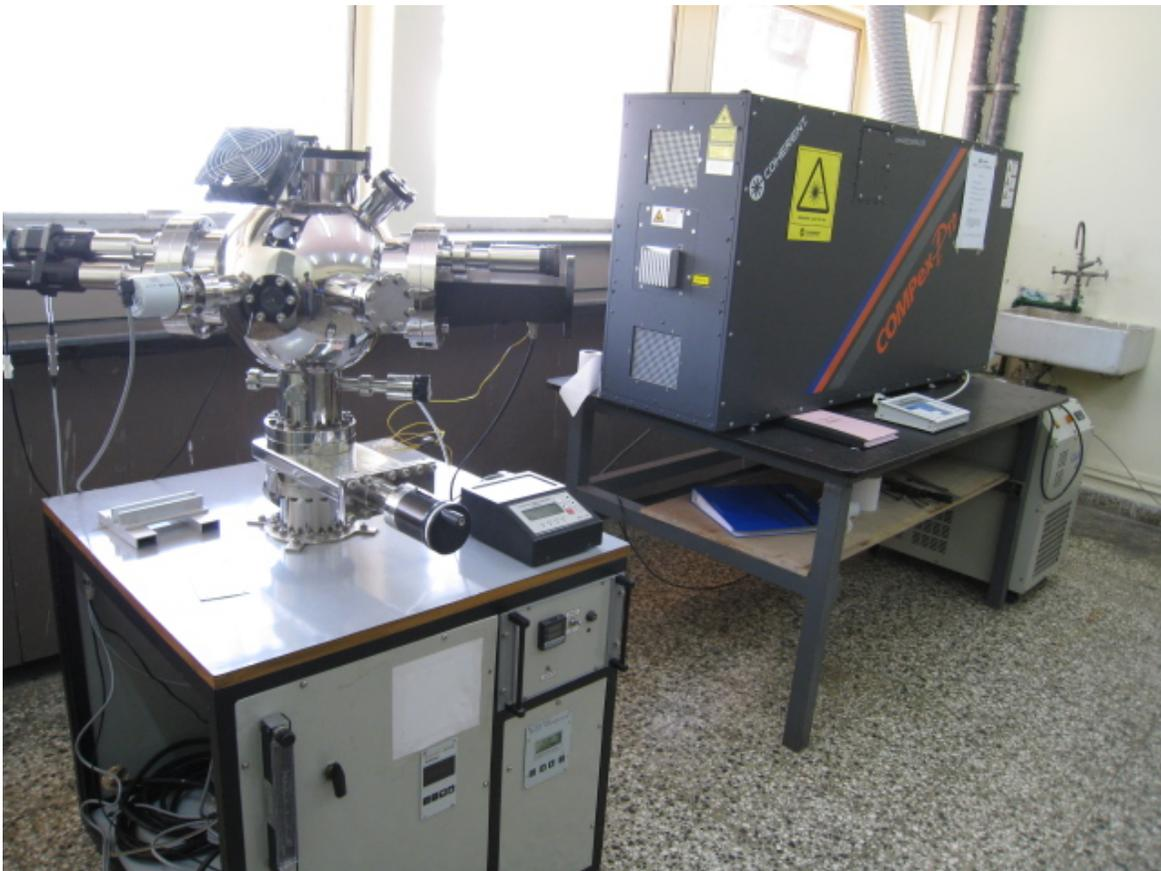
**Fig. 2.3:** Photograph of the PLD system.
