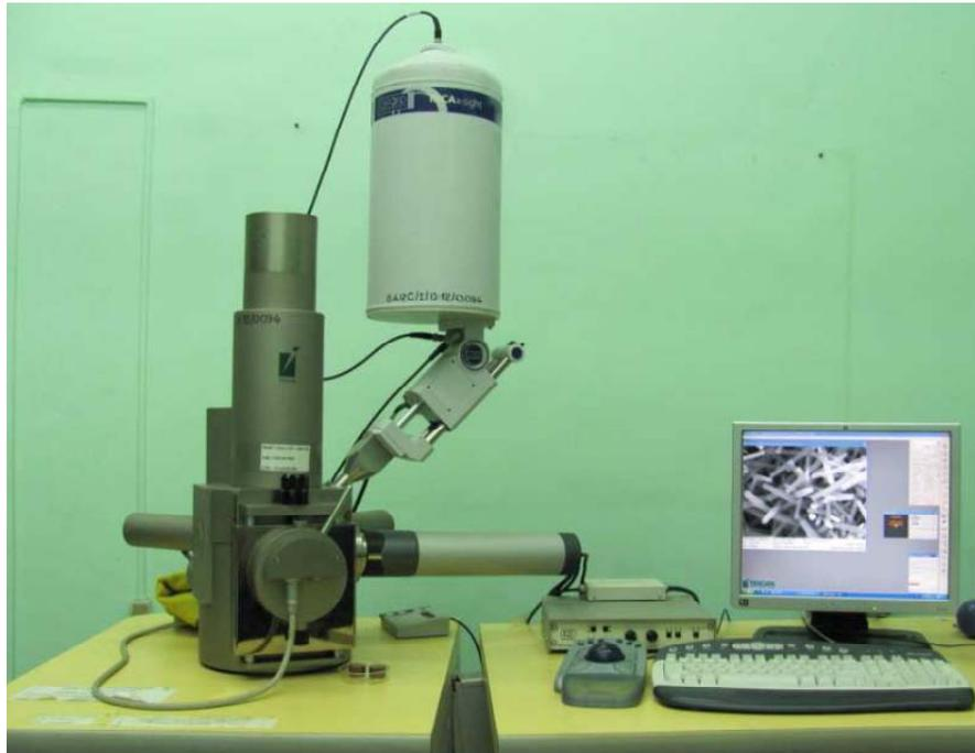
**Fig. 2.10:** Photograph of SEM (model: Tescan VEGA MV2300T/40).
