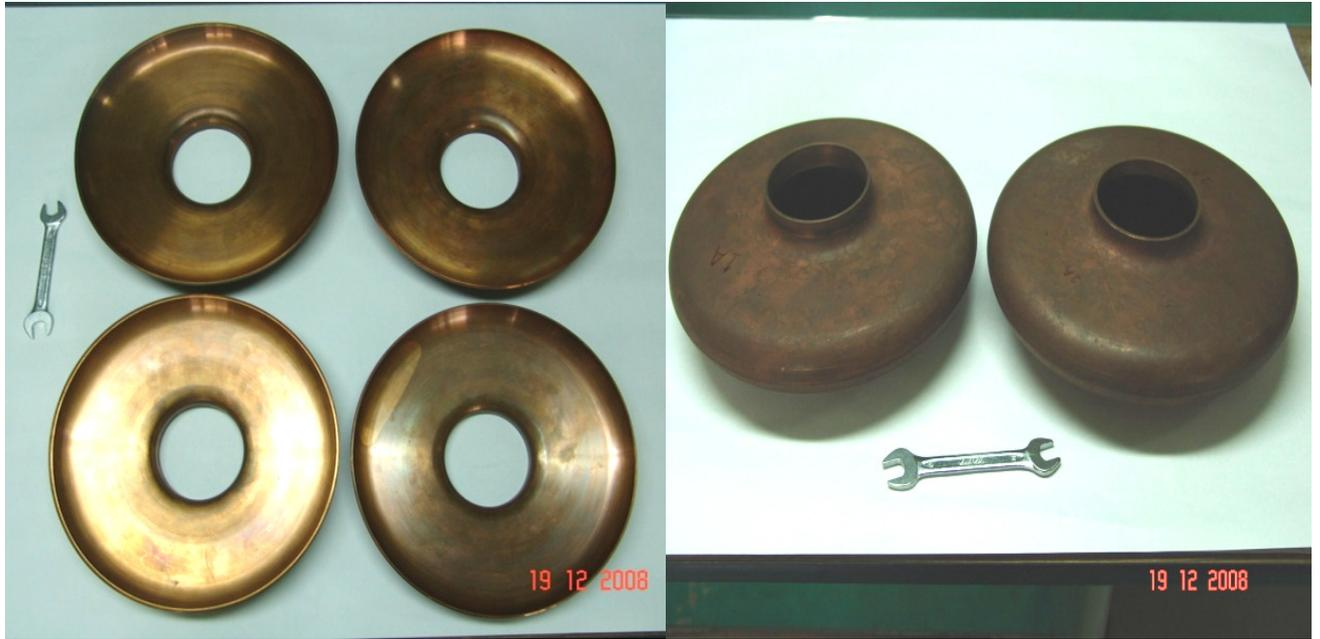
Figure 39: Formed Copper cavities ( $f = 1.05$  GHz); photographs showing half cells and full cells
