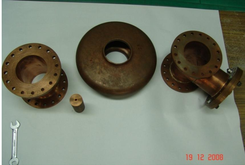
Figure 26: Cavity, Beam pipe and Coupler Parts
