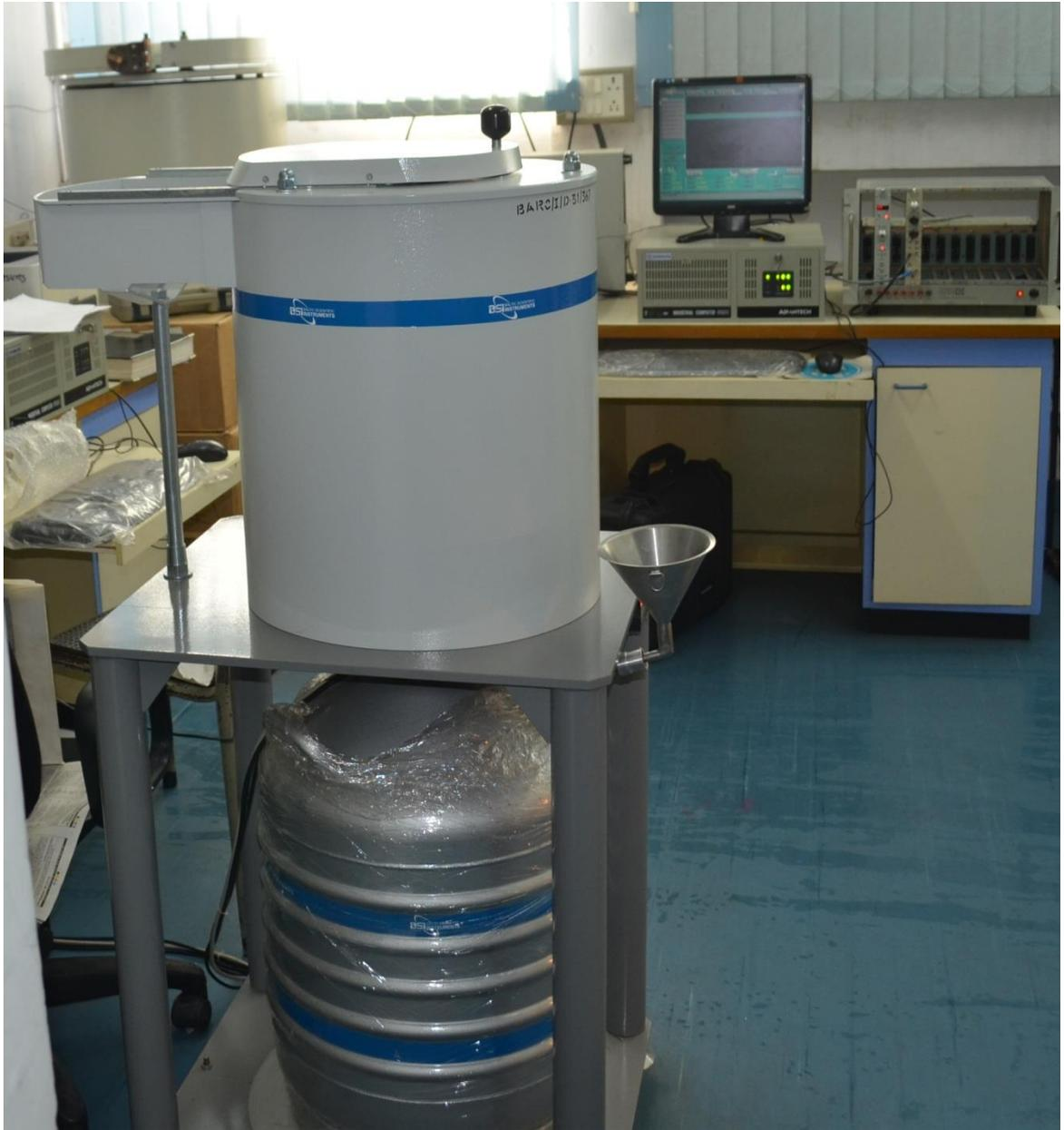
**Figure 3.1 HPGe Gamma Spectrometry system in the Low Level Counting Lab**
