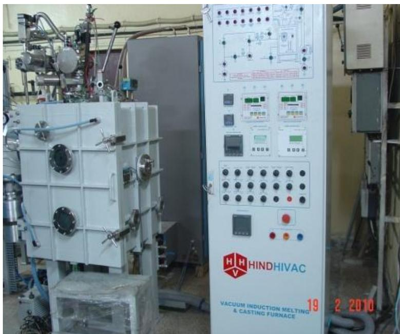
*Figure 1.9. Inductively heated vacuum melting system*
