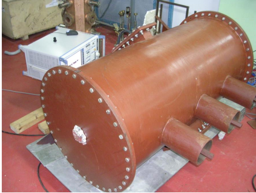
Fig. 5.4. Frequency measurements on the DTL prototype.
