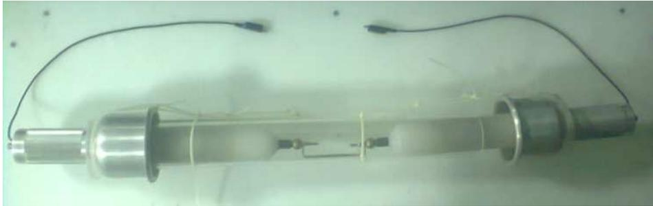
Figure 2.5: Cascaded High Voltage Probe
