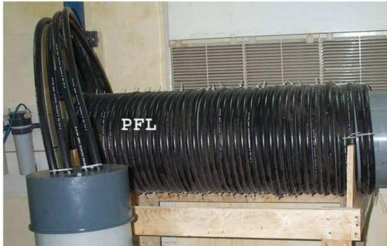
Figure 3.1: Pulse forming line made of RG218 cable
