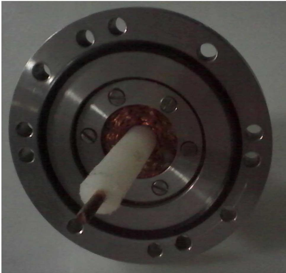
Figure 3.4: RG218 cable with connector for fitting
