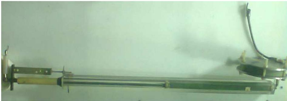
Figure 2.1: Resistive Voltage Divider
