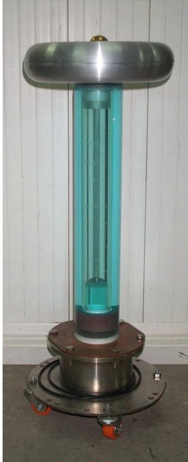
Figure 2.3: High BW Resistive Voltage Divider
