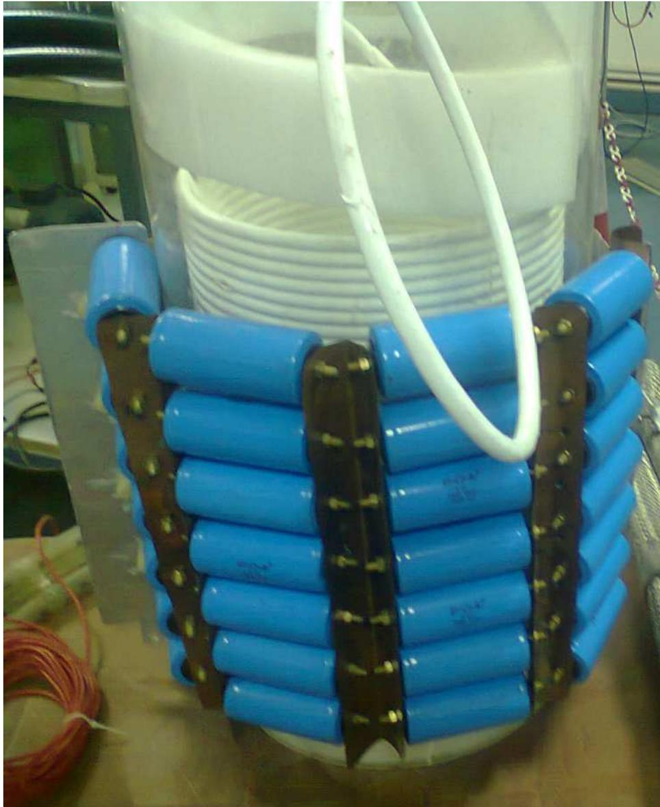
Figure 4.8: High Voltage Pulse transformer
