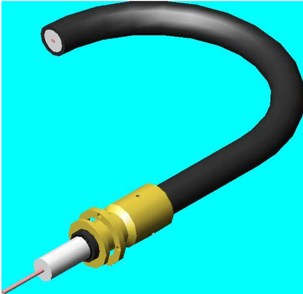
Figure 3.6: High voltage XLPE cable with connector for fitting
