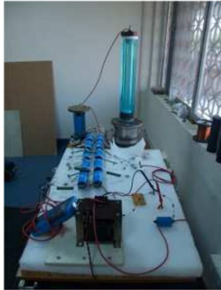
Figure 7.2: Experimental Setup with Marx generator
