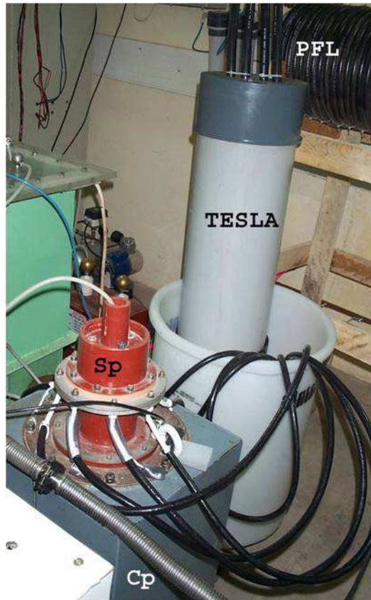
Figure 4.1: Primary capacitor and pulse transformer for experiments of first set
