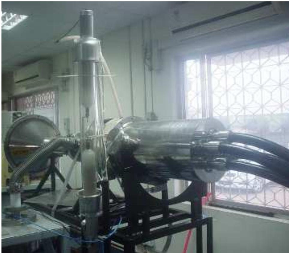
Figure 6.21: Picture of virtual cathode oscillator assembly fitted with the cable based PFL
