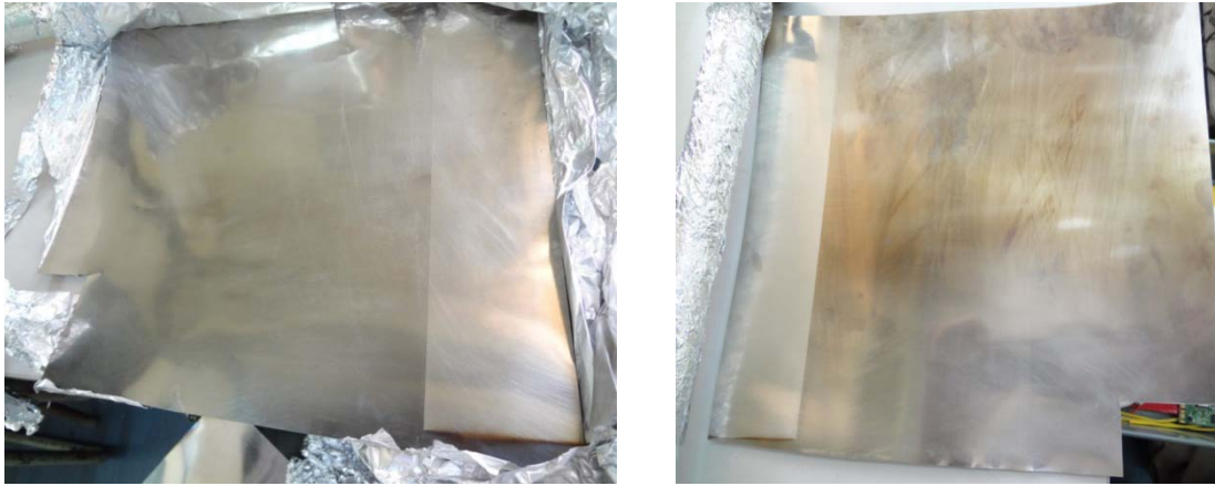
Fig. 2.16: Different types of substrate on which NEG film have been deposited.
