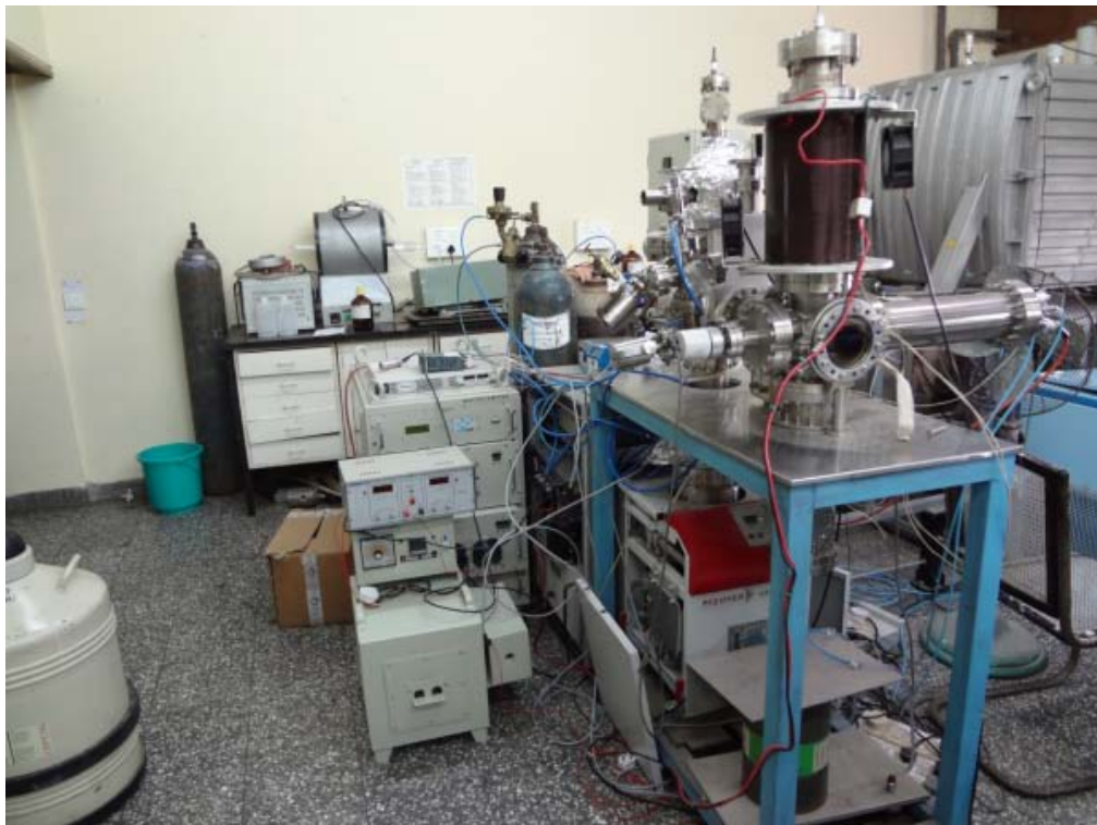
Fig.2.8: Photograph of the DC-magnetron sputtering system showing pumps and electronic instruments.
