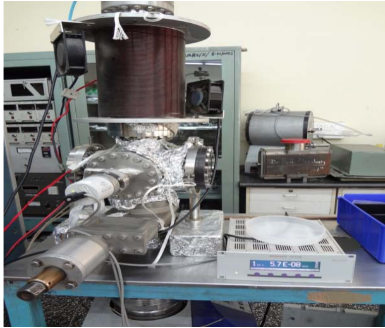
Fig. 2.9: Photograph of DC-magnetron sputtering system showing a base pressure of 5.7 \times 10^{-8} mbar.
