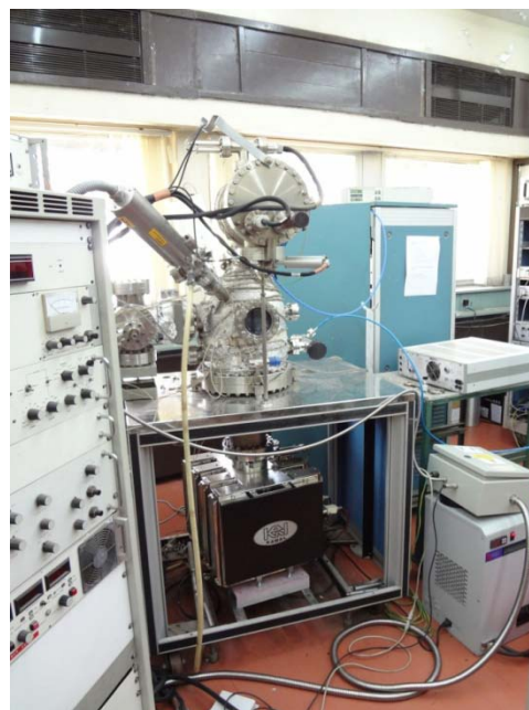
Fig.3.5: Photograph of our XPS system.
