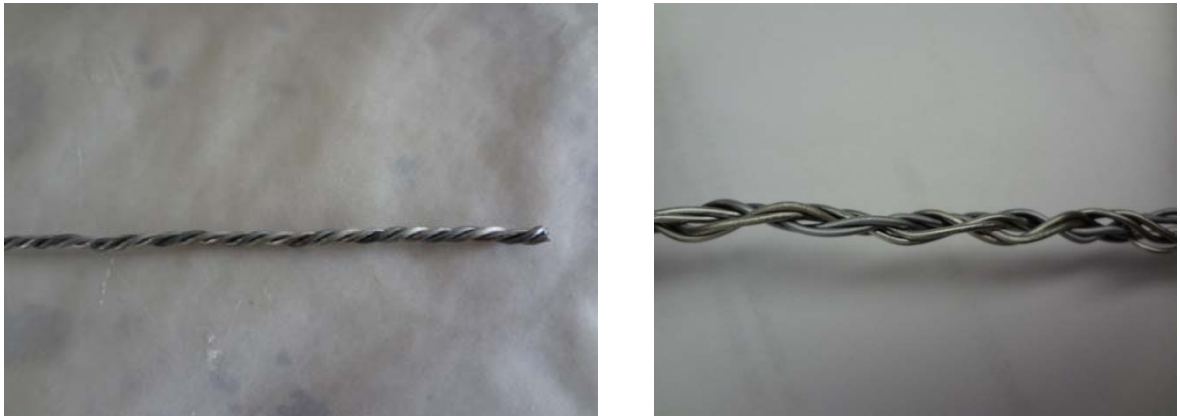
Fig. 2.15: Different types of inter-twisted ternary targets of (Ti-V-Zr) used in sputtering system.
