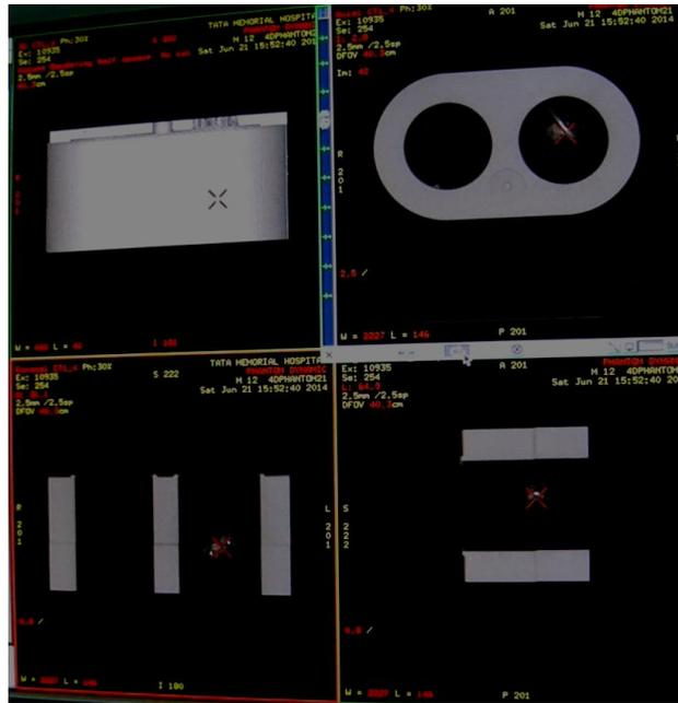
**Figure 7.10:** Screenshot captured during motion of target and showing displacement of copper marker placed inside the target in different section.
