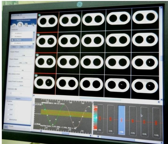
**Figure 7.8:** Screenshot showing sorted images of the phantom at 30% phase and associated motion pattern.
