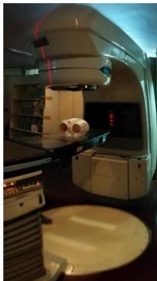
**Figure 4.12:** Photograph showing setup of IMRT audit phantom.
