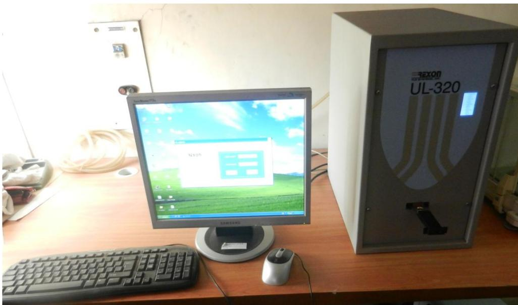
**Figure 4.9:** Photograph of computerised TLD reader system used in this work
