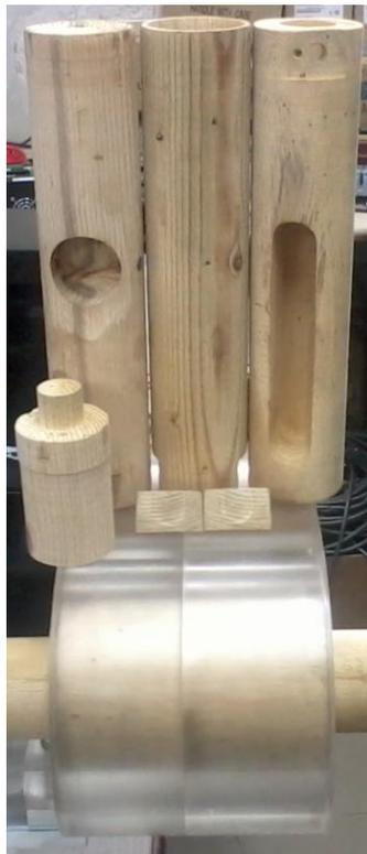
**Figure 7.2:** Photograph of some of the inserts available with the dynamic phantom.
