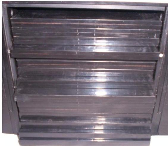
**Figure 3.2(c):** Photograph of radiochromic film holder.
