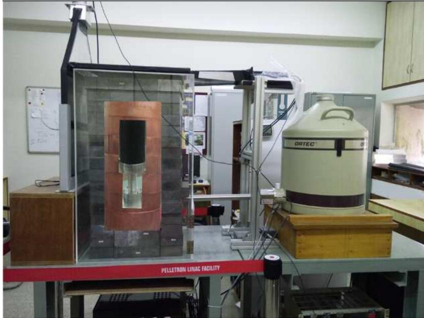
Figure 3.8: A picture of the TILES with complete shielding arrangement.
