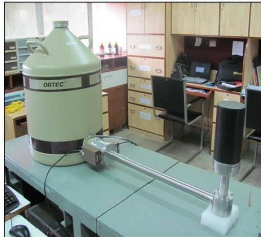
Figure 2.1: The low background HPGe detector (ORTEC GEM75-95-LB-C-HJ).
