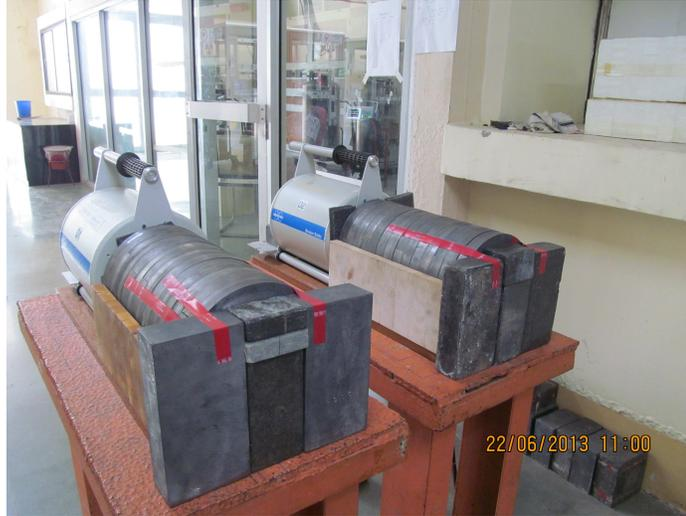
Figure 4.2: A picture of the HPGe detectors D1 and D2 with 5 cm normal Pb shield.
